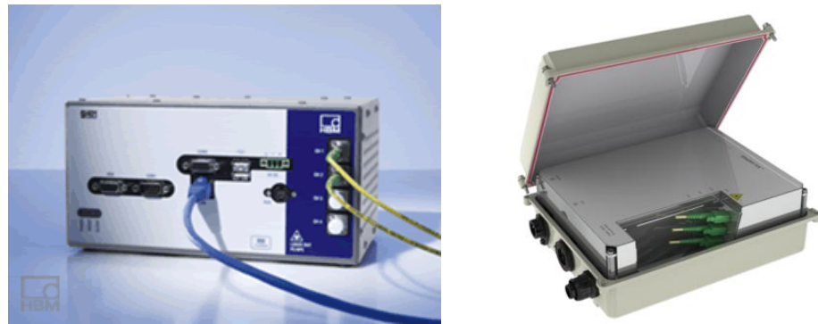
Figure 4.1: Interrogators as used in the field tests: HBM (left) and FibreSensing (right)
