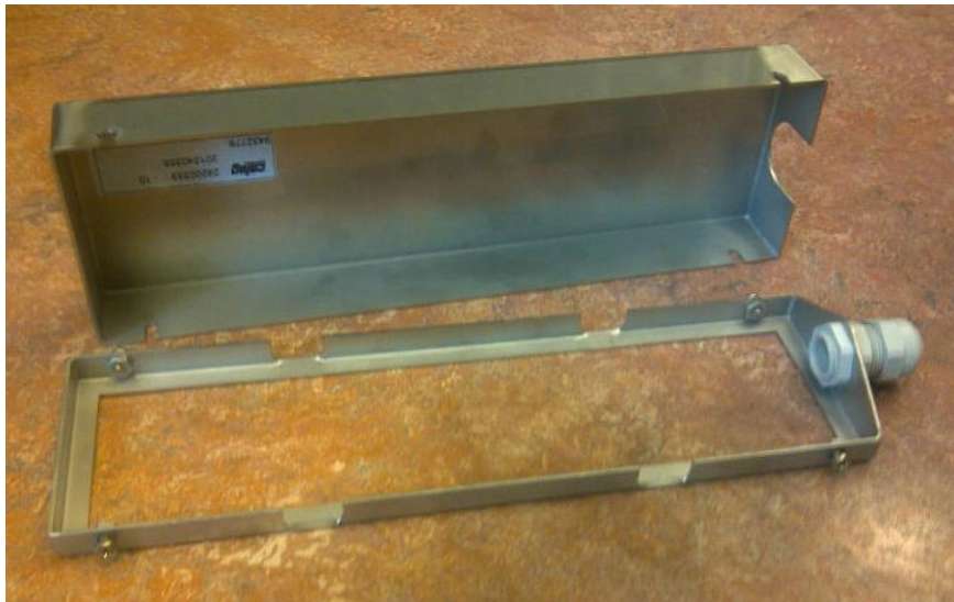
Figure 6.2: New protection box design to allow easier access to the assembly with its screws and connectors. The re-design was based on the field tests carried out in the Nordex N80 turbine;
