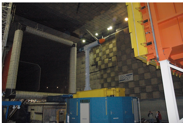
Figure 4.2 Setup of model turbine in the Measurement Section of the DNW LLF
