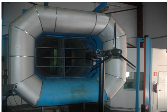
Figure 10.5 Outline of INTA's wind tunnel experiment
