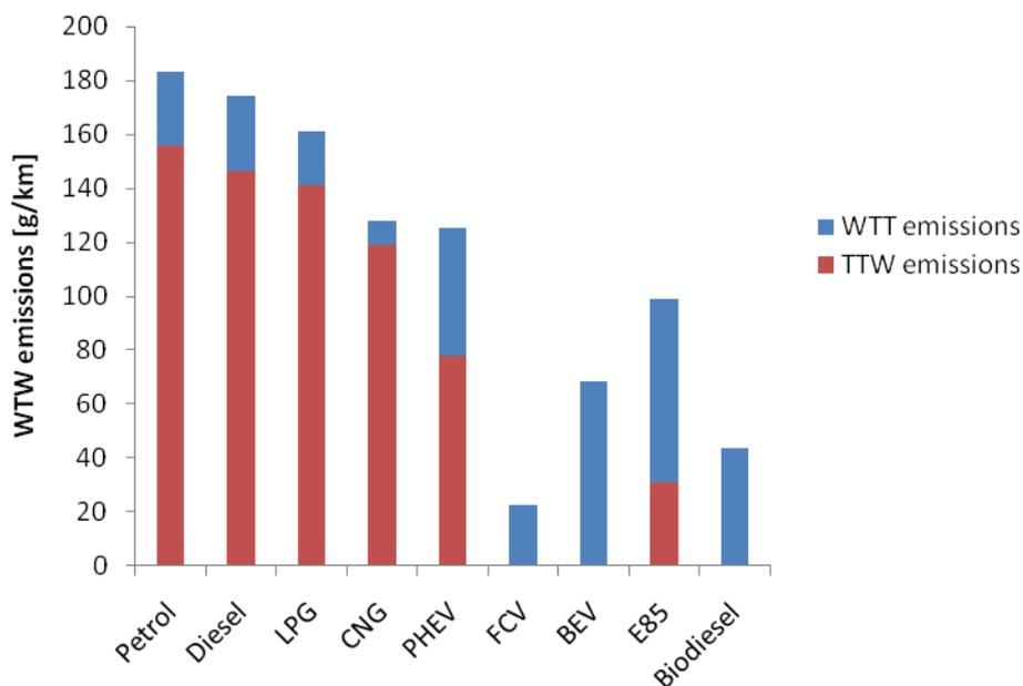
Figure 2.1 *WTW-emissions of different vehicle-fuel combinations*
