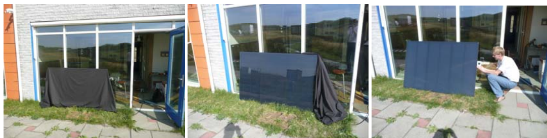
Figure 4.1 Outdoor test of HV CIS module [ECN]
