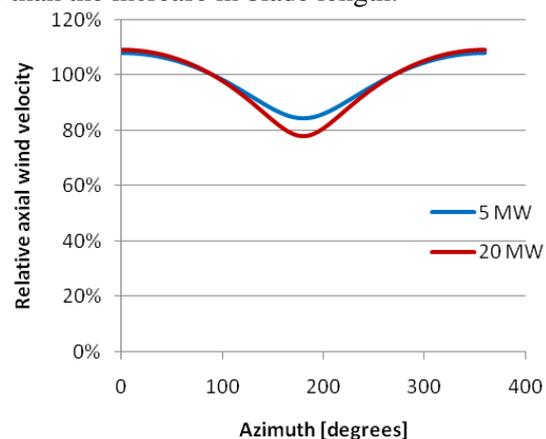
Figure 6.1 *Wind shear is stronger for a relatively shorter tower*
