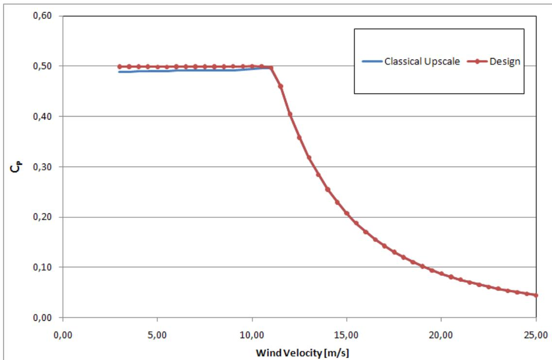
Figure 3.14  $C_p$  performance of the 20MW design for different wind speeds compared with the  $C_p$  of the 20MW upscaled wind turbine
