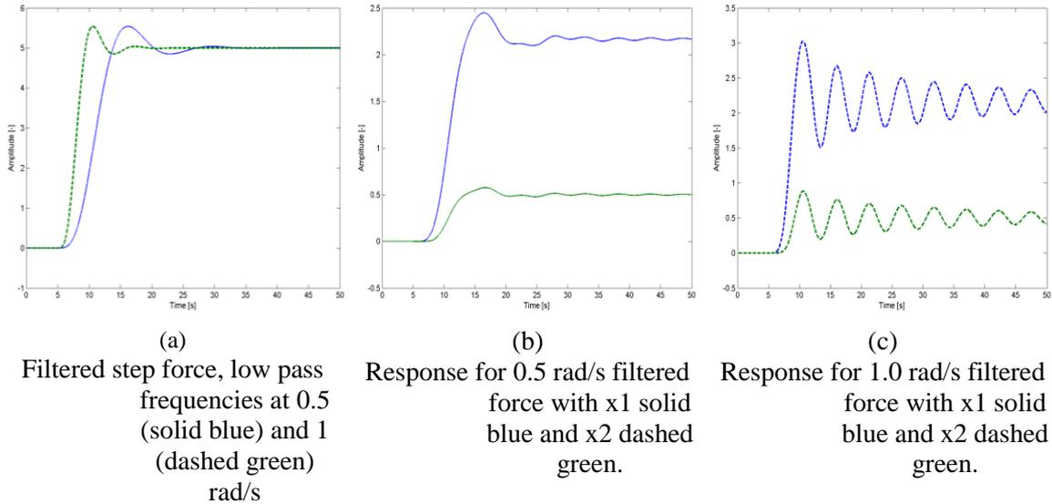
Figure 5.2 Disturbances and according responses of a mass-spring damper system
