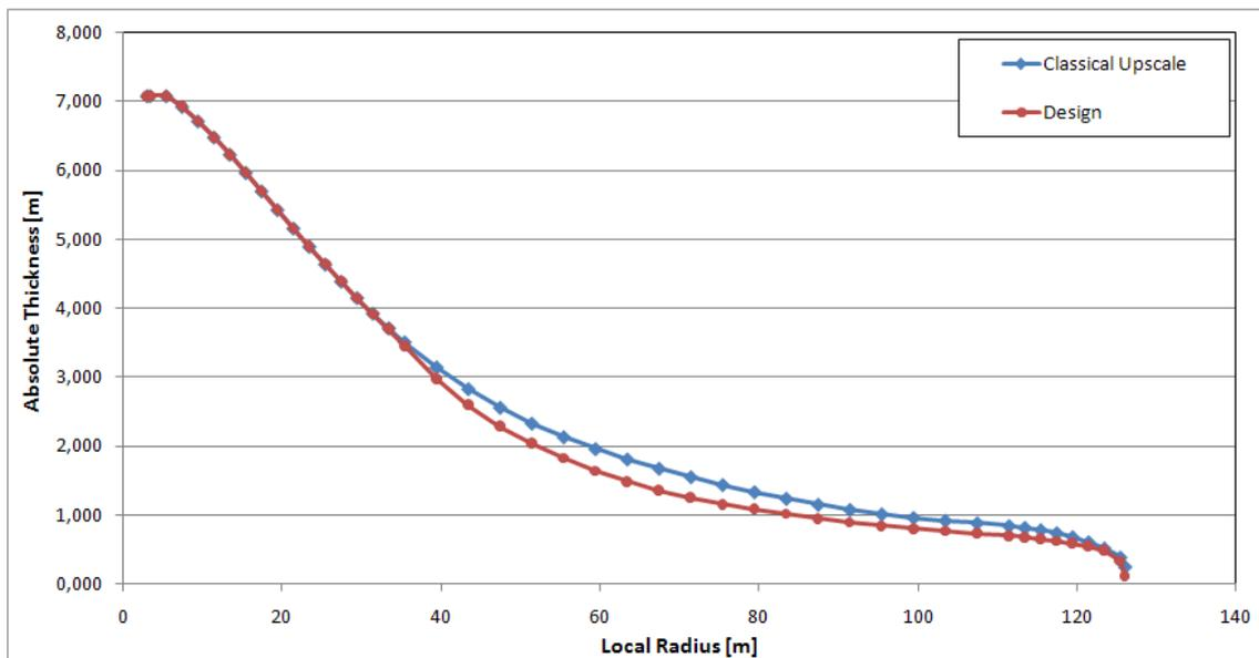
Figure 3.10 20MW wind turbine design absolute thickness distribution compared with the upscaled 20MW absolute thickness distribution.
