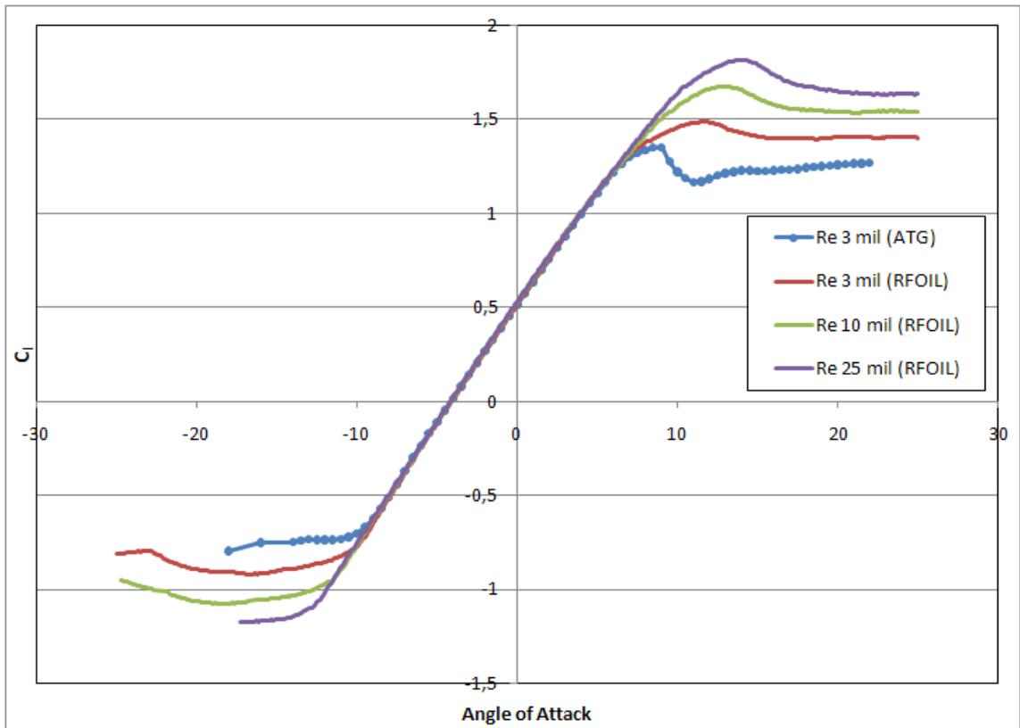
Figure 3.4  $C_l$  versus Angle of Attack curve of DU93-W-210 airfoil for different Reynolds numbers
