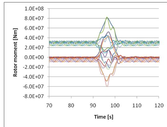
Figure 5.12 Rotor moments for extreme wind shear conditions, 20 MW turbine
