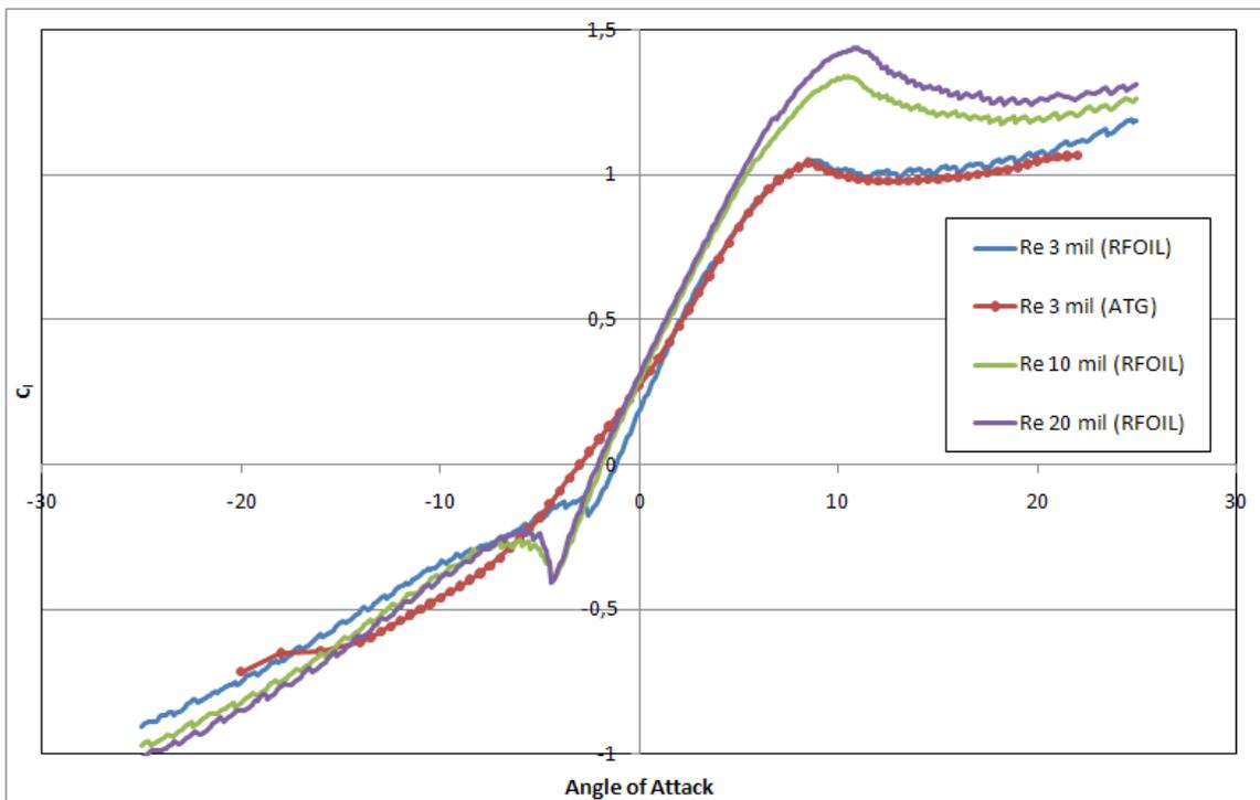
Figure 3.6  $C_l$  versus Angle of Attack curve of DU00-W2-401 airfoil for different Reynolds numbers
