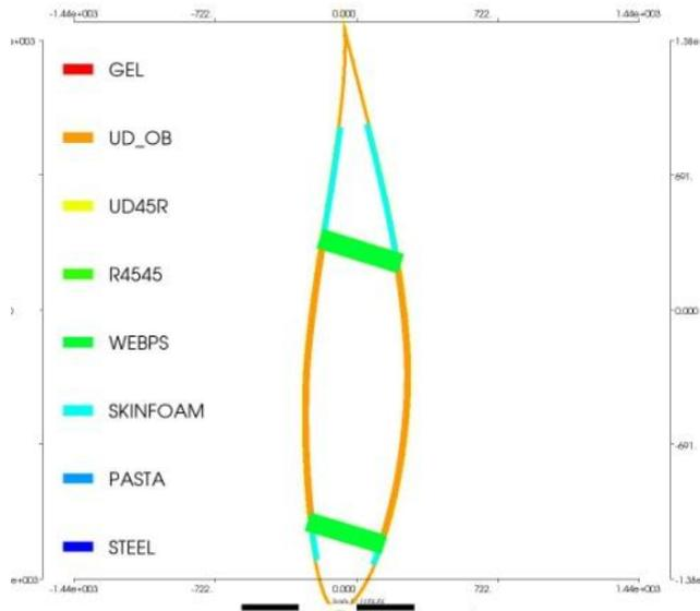
Figure 4.11 Cross section at 118 m
