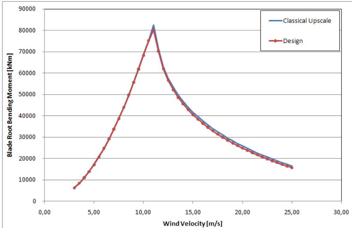
Figure 3.15 Blade root bending moment of the 20MW design compared with the 20MW upscaled wind turbine for different wind speeds
