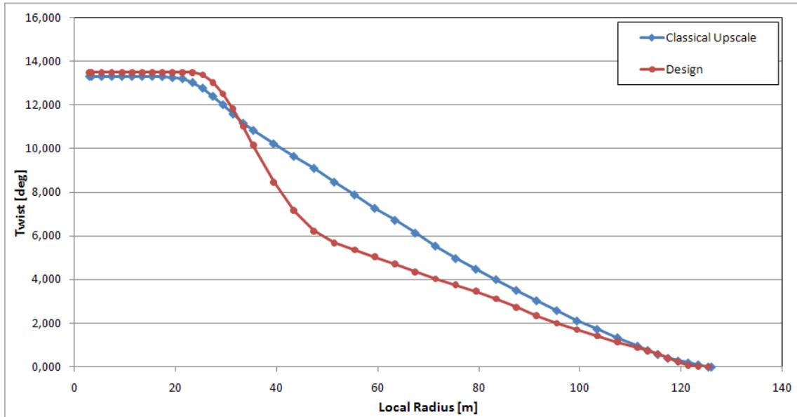
Figure 3.9 20MW wind turbine twist distribution compared with the upscaled 20MW twist distribution
