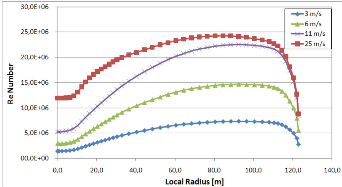
Figure 3.1 Reynolds number distribution along the blade for different wind speeds
