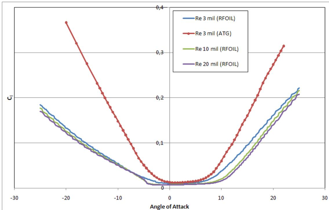
Figure 3.7  $C_d$  versus Angle of Attack curve of DU00-W2-401 airfoil for different Reynolds numbers
