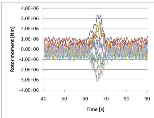
Figure 5.11 Rotor moments for various extreme wind shear conditions, 5 MW turbine
