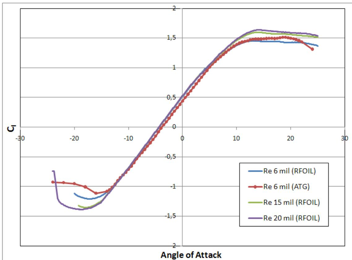
Figure 3.2  $C_l$  versus Angle of Attack curve of NACA 64-618 airfoil for different Reynolds numbers
