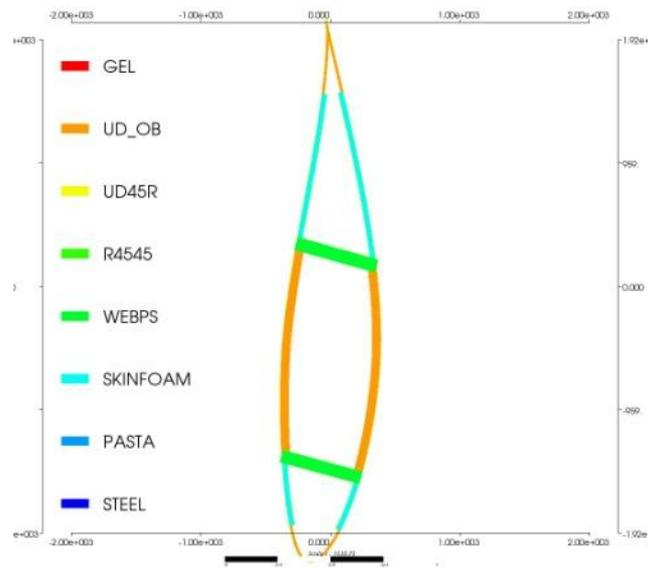
Figure 4.10 *Cross section at 100.4 m*
