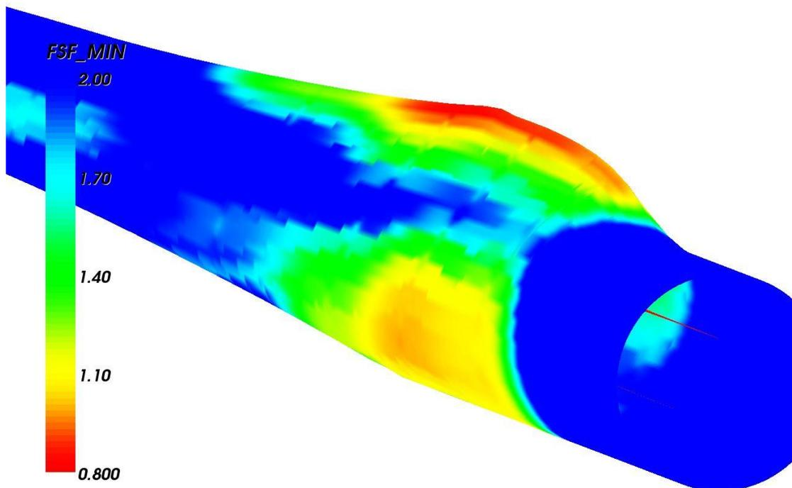
Figure 6.2 *Fatigue Safety Factor (FSF) on blade.*
