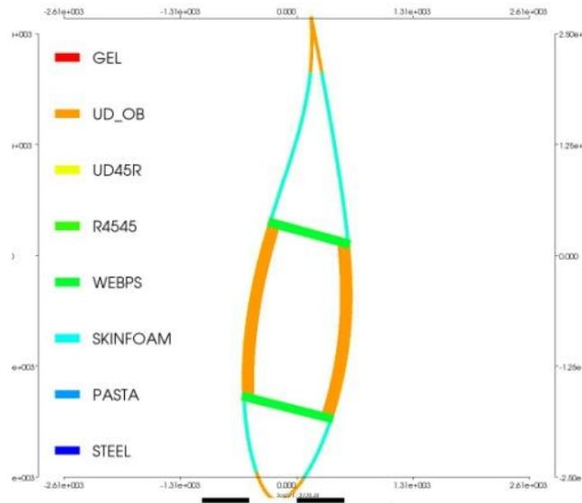
Figure 4.9 *Cross section at 71 m*
