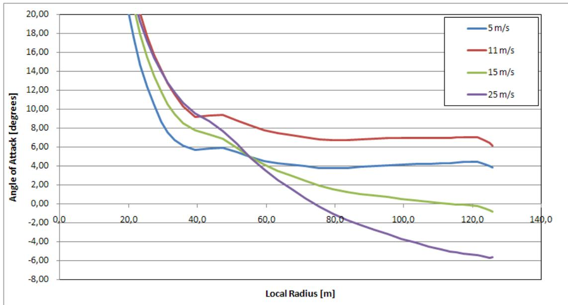
Figure 3.11 Local angle of attack distribution along the blade span for different wind speeds.
