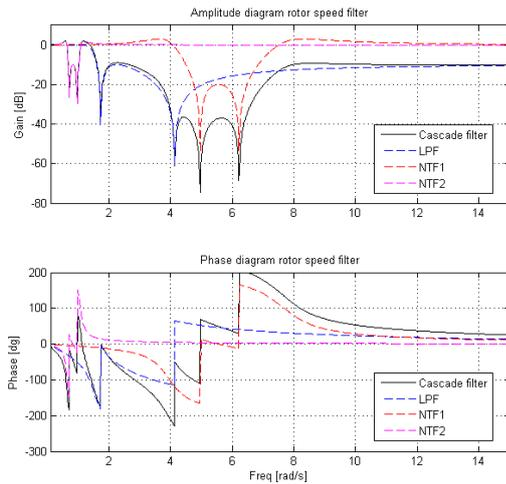
Figure 5.6 Rotor speed filter of the controller for the 20MW turbine
