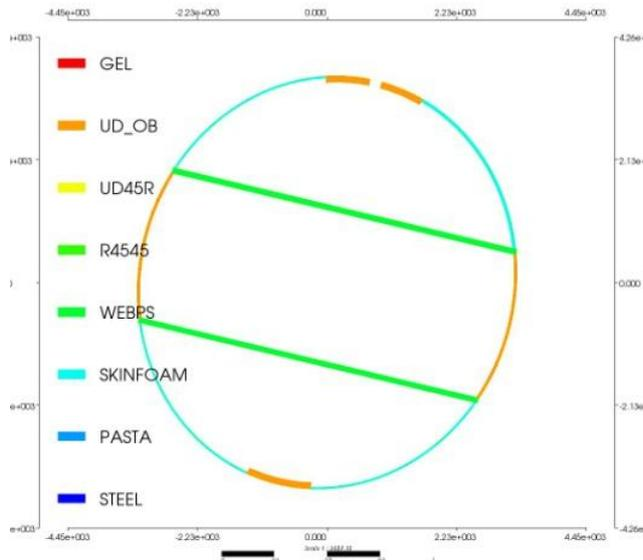
Figure 4.3 Cross section at 8.4m
