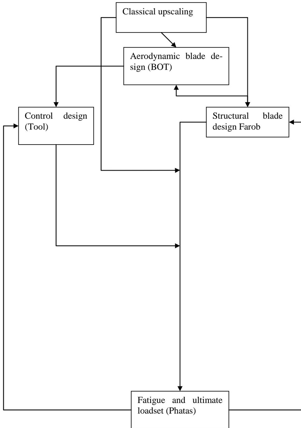
Figure 2.1 *Flow diagram of design process.*
