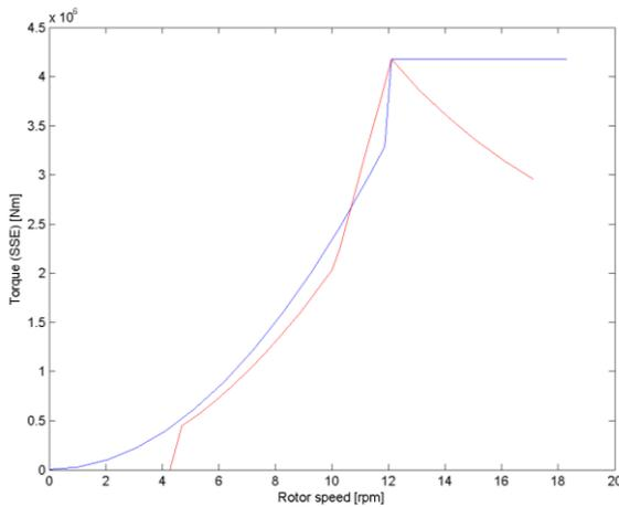
Figure 5.4 *Qn* curve for the reference 5MW turbine as designed originally (blue) and the new design (red)
