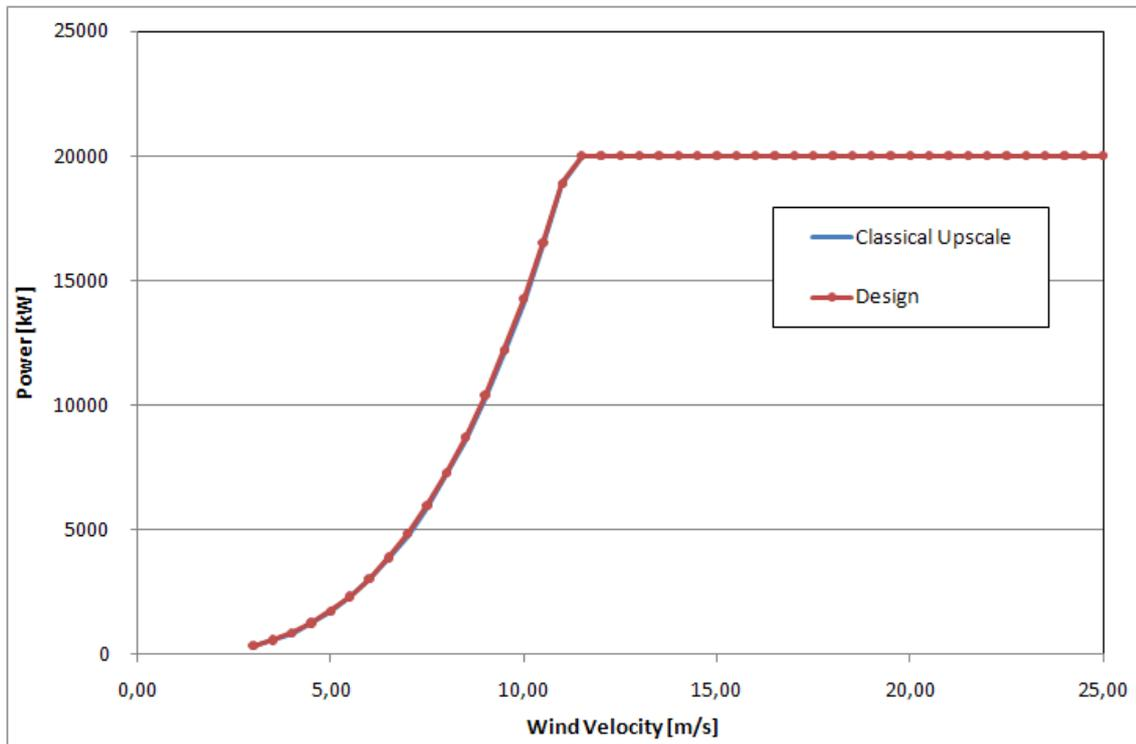
Figure 3.13 The power production of the 20MW design for different wind speeds compared with the 20MW upscaled wind turbine
