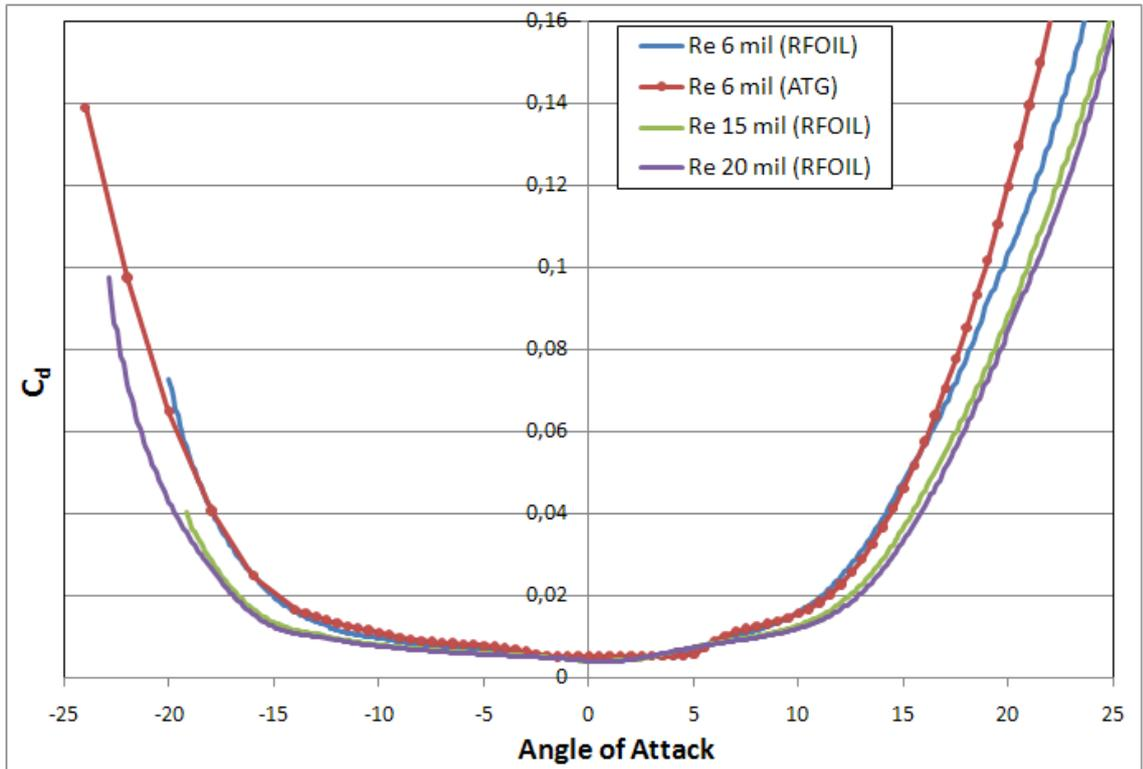
Figure 3.3  $C_d$  versus Angle of Attack curve of NACA 64-618 airfoil for different Reynolds numbers
