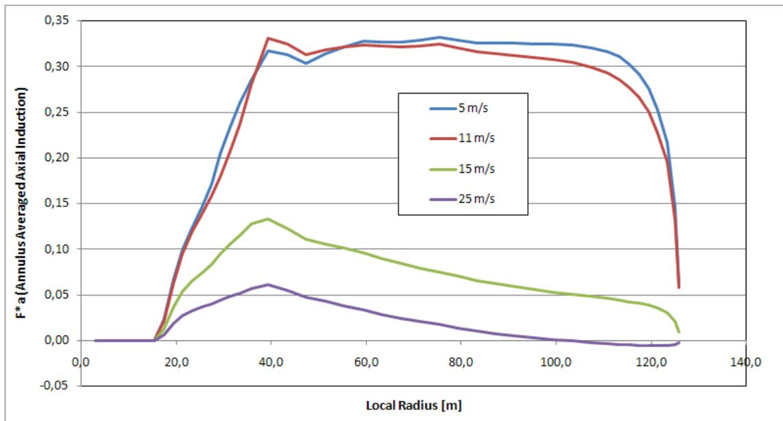
Figure 3.12 Axial induction distribution along the blade span for different wind speeds.
