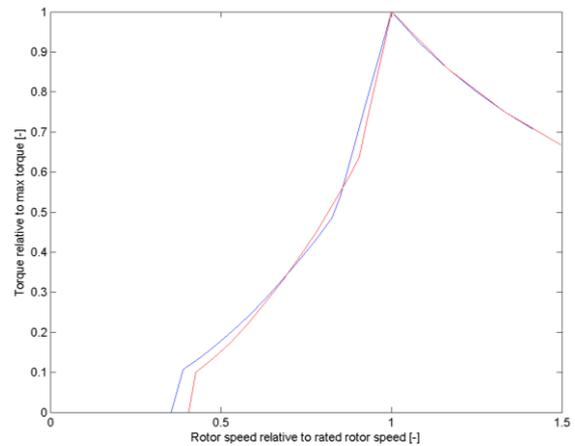
Figure 5.5 Normalised *Qn* curves as designed for the 5 MW reference turbine (blue) and the 20 MW turbine (red)
