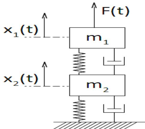
Figure 5.1 A simple mass spring system
