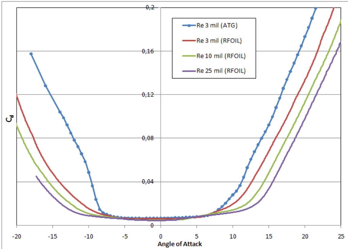
Figure 3.5  $C_d$  versus Angle of Attack curve of DU93-W-210 airfoil for different Reynolds numbers
