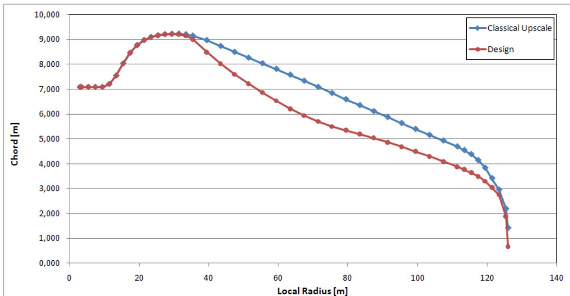
Figure 3.8 20MW wind turbine chord distribution compared with the upscaled 20MW chord distribution
