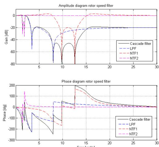
Figure 5.3 Rotor speed filter of the controller for the 5MW controller
