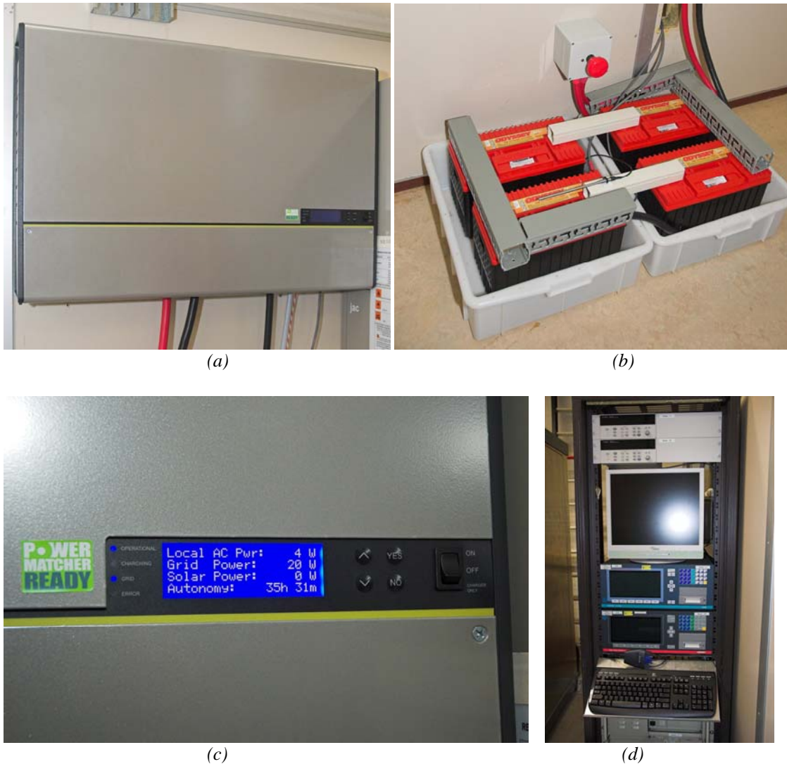
Figure 3.1 Photos of the test set-up. (a) the Atrium, (b) the lead-acid batteries, (c) close-up of the Atrium display and (d) the data acquisition equipment
