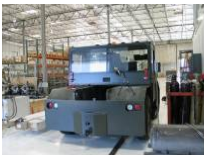
Figure 94: NMC-Wollard Tow Tractor Powered with Lynntech Fuel Cell
