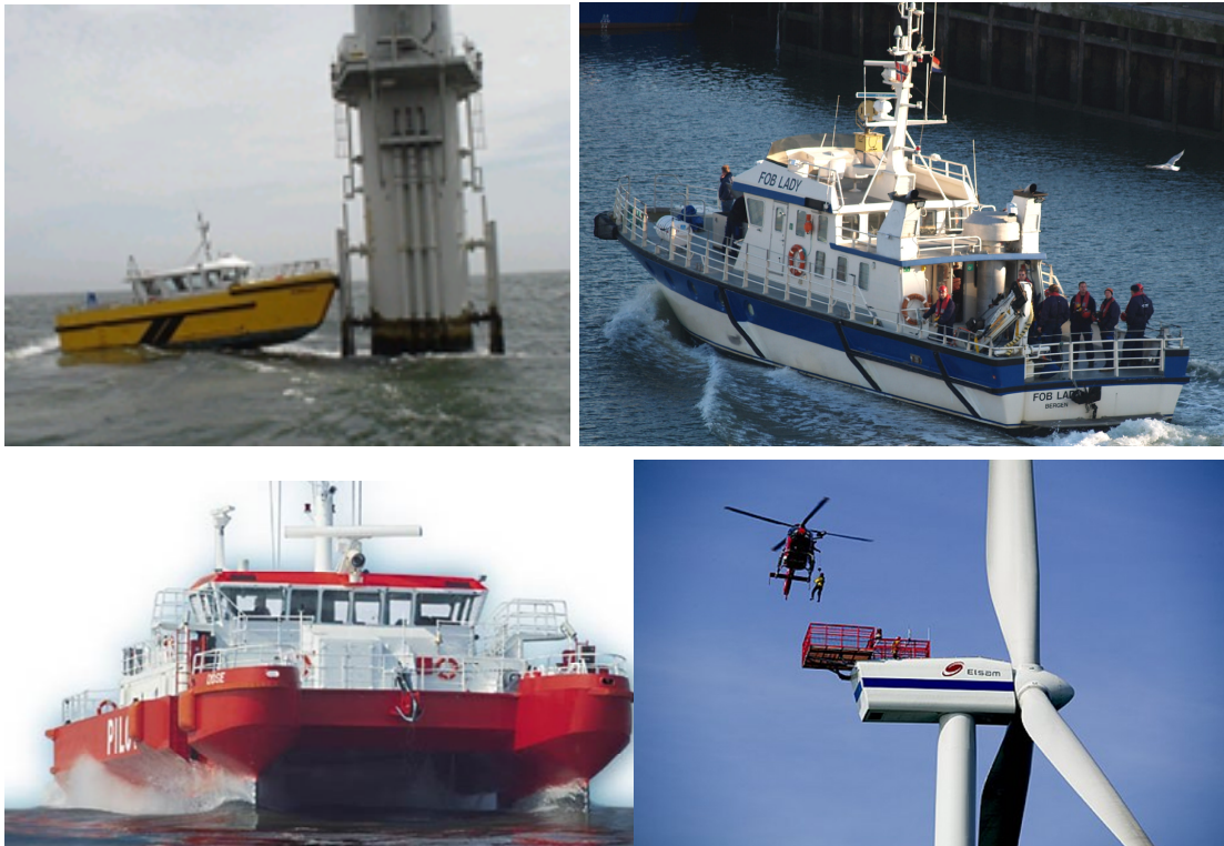
Figure 2.3: Examples of transportation and access equipment for maintenance technicians; clockwise: Windcat workboat, Fob Lady, helicopter, and SWATH boat
