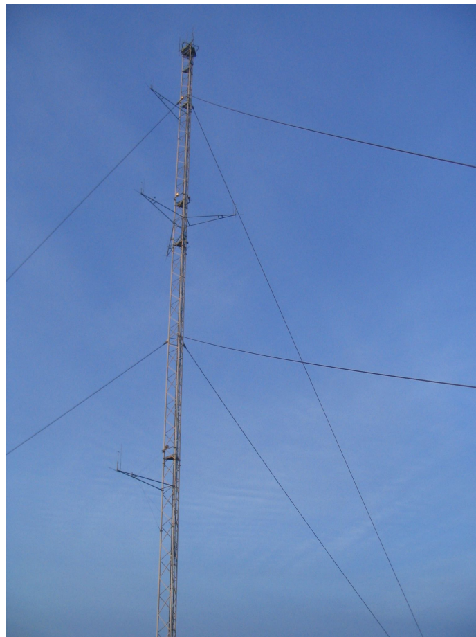
Figure 3.2 View of the meteorological mast 2 with attached booms at different levels. The booms at the upper and lower levels are positioned at 78.5m and 24.2m heights and are directed to 215° with respect to North.
