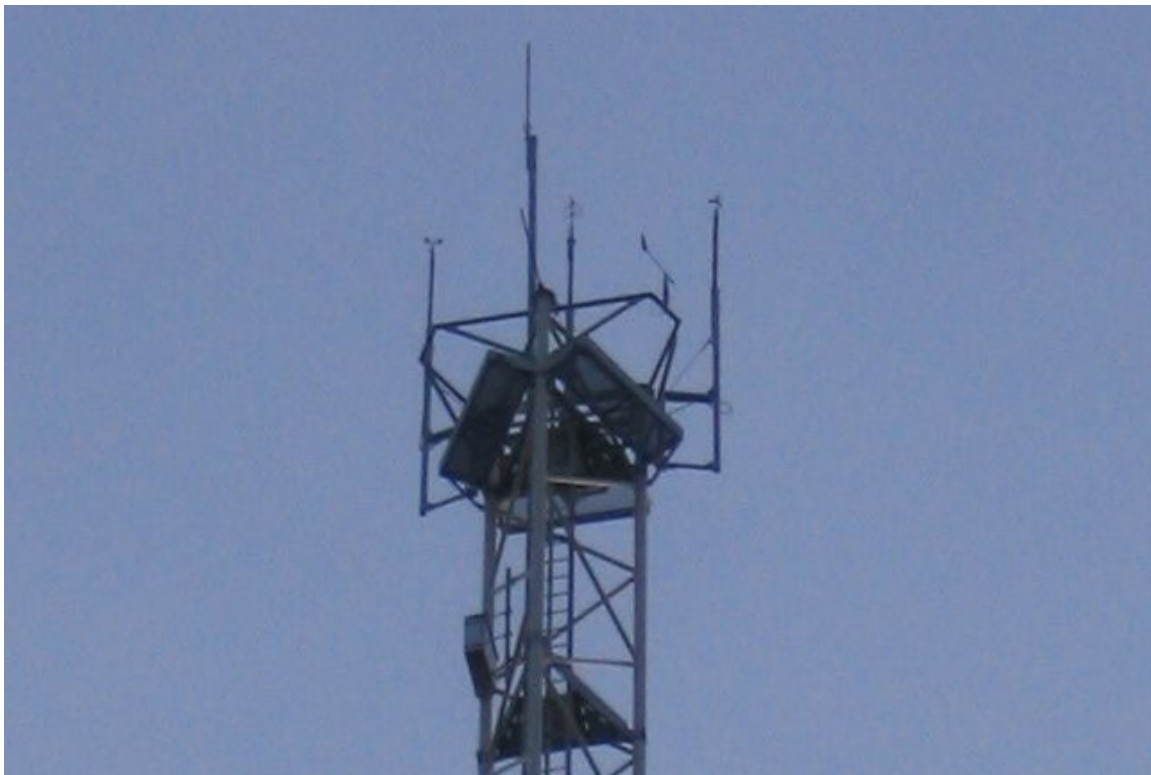
Figure 4.3 Top of the meteorological mast 2 with 3D sonic sensor, 2 cup anemometers, 2 wind vanes aviation warning light and lightning conductor. The boxes lower in the mast contain the signal connection and high voltage protection.
