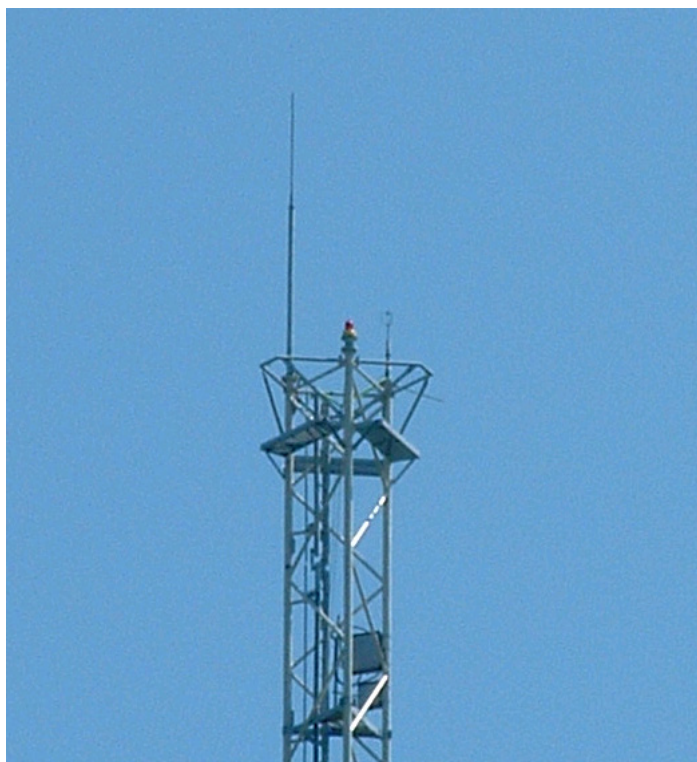
Figure 4.1 Top of the meteorological mast 1 with 3D sonic sensor, wind vane, aviation warning light and lightning conductor. The boxes lower in the mast contain the signal connection and high voltage protection.
