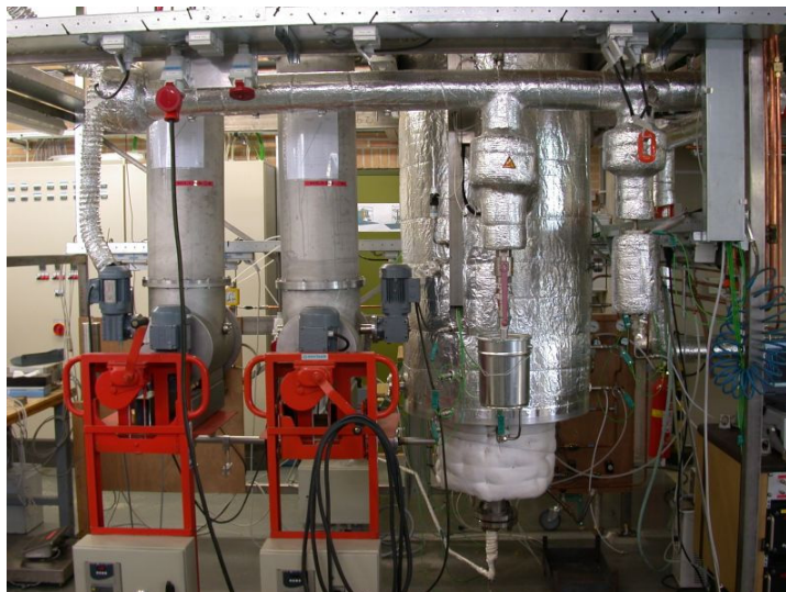
Figure 3.5 Lab-scale 5 kg/h MILENA gasifier at ECN
