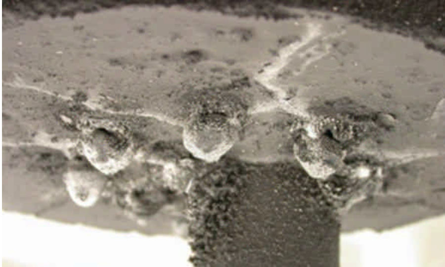
Figure 3.3 Deposits on upstream side of gas distributor plate of HELGA cooler (test 1)
