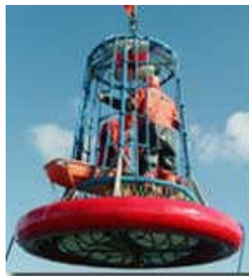
Fig. 4.2: Basket to hoist personnel from the vessel to the turbine
