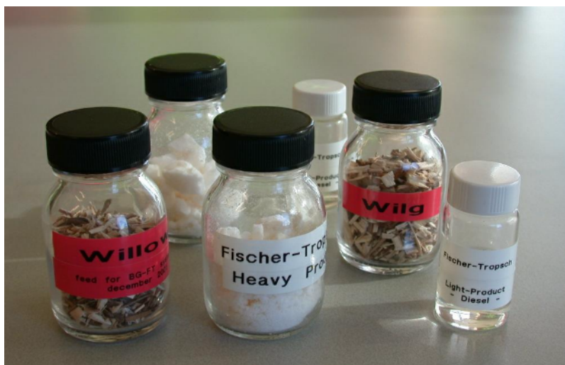
Figure 6.2. Pictures of the willow used for the integrated test in December 2001, Fischer-Tropsch wax, and the light product (viz. 'green diesel').
