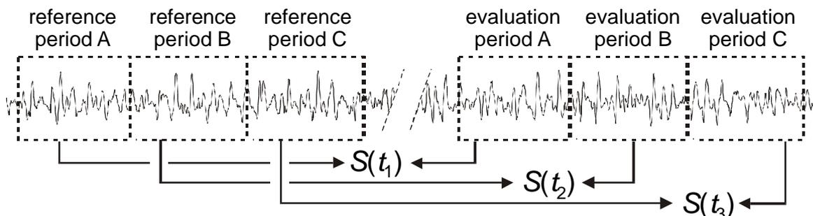
Figure 3.15 Example of the moving reference method. The  $S$ -value is obtained by comparing the attractors of a moving reference period with attractors from evaluation pressure time series. Both windows progress in time from A to B to C etc. The time delay between the reference and evaluation time window is constant.
