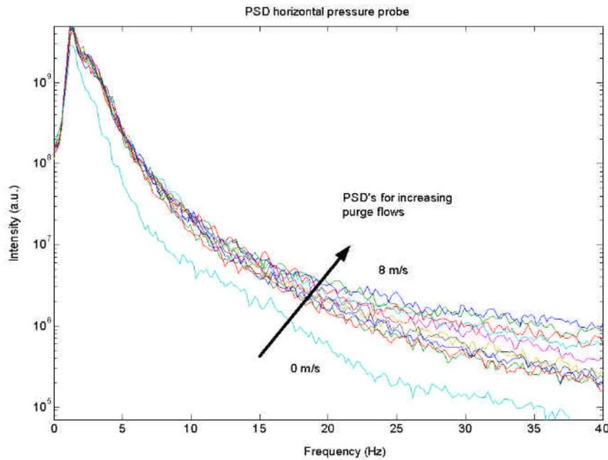
Figure 2.4 Example PSD analysis of pressure fluctuation measurements at varying purge flows.
