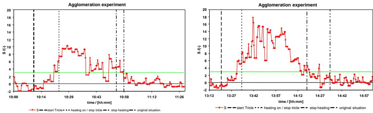
Figure 2.12 *Agglomeration experiments with a bed of 3.6 kg and water flow rate of 6.5 ml/min. Both experiments illustrate the recovery from an agglomeration warning.*
