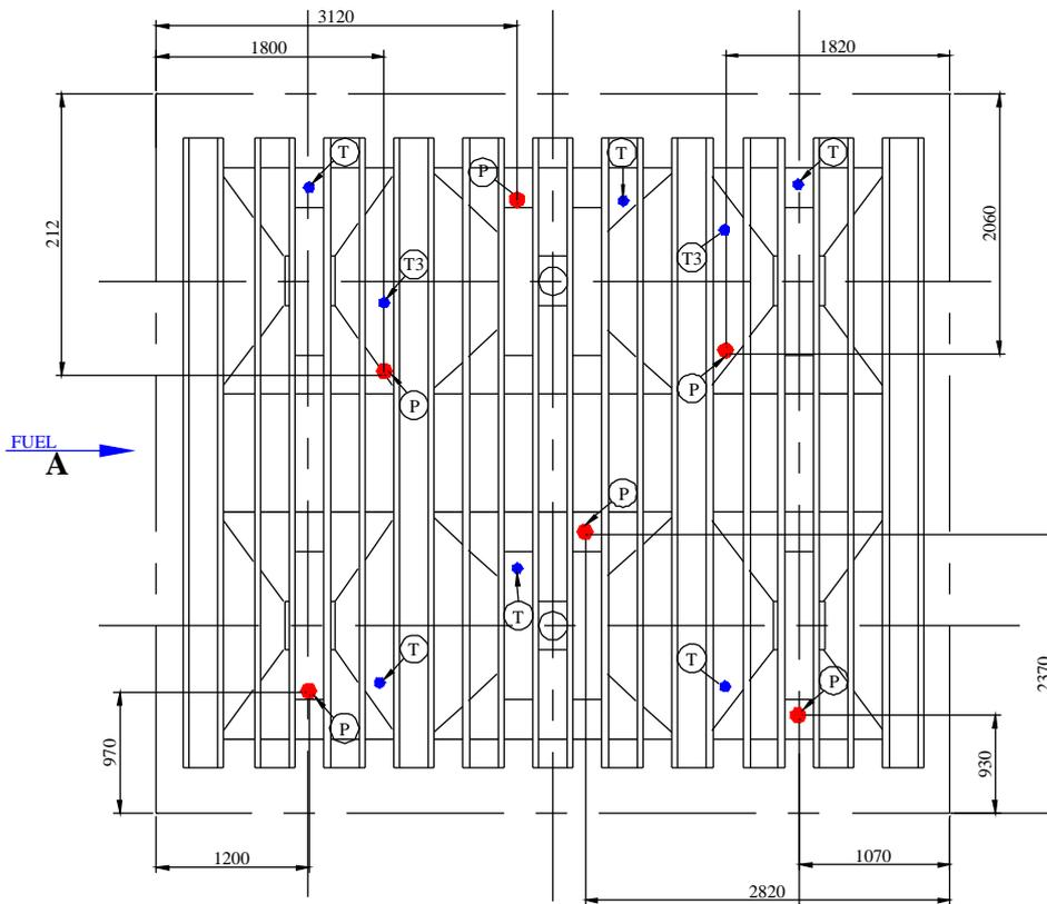
Figure 3.2 Pressure fluctuation measurement probes in 80 MW<sub>th</sub> fluidised-bed combustor: location of six probes (red circles).
