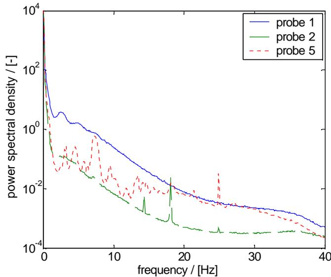
Figure 3.25 The power spectra for pressure signals measured at three locations during the test week.
