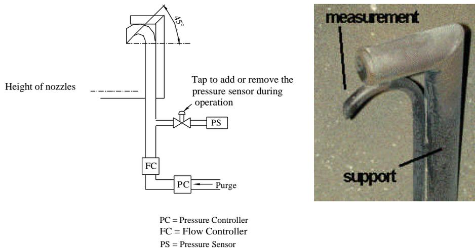
Figure 3.1 *Set-up of the probe for pressure measurements. To the right: photo of initial design for the 80 MW<sub>th</sub> fluidised-bed combustor.*
