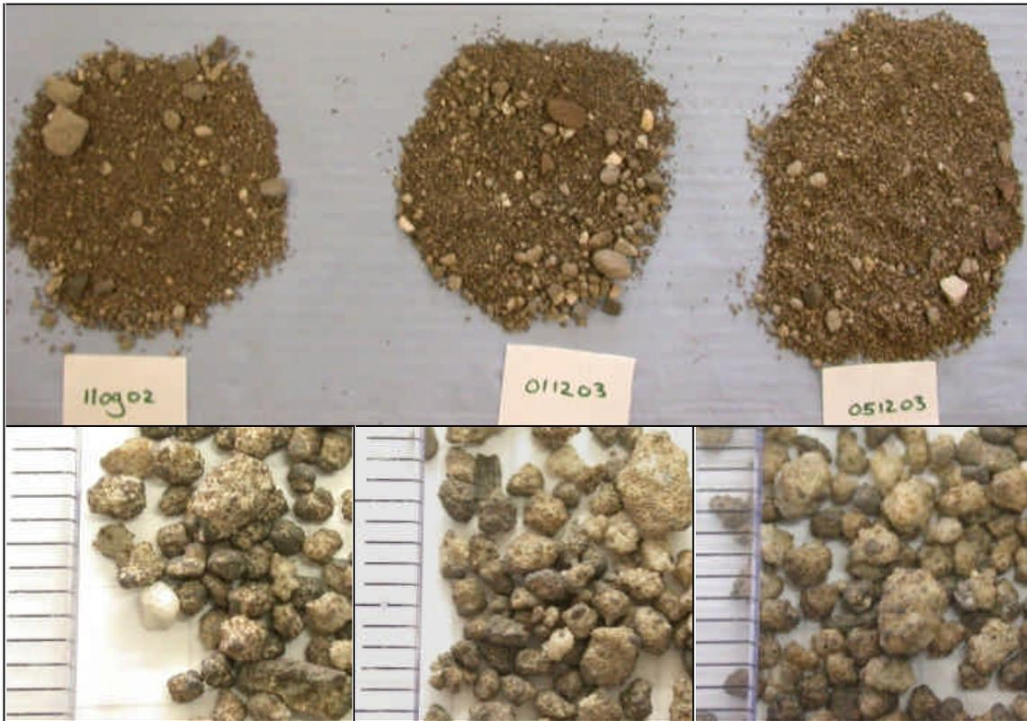
Figure 3.24 Photos of bed material from the BFB combustor (only particles  $>1200 \mu\text{m}$ ). Left: 11.09.2002 sample (reference); middle: 01.12.2003 sample (start of test week); right: 05.12.2003 sample (end of test week).
