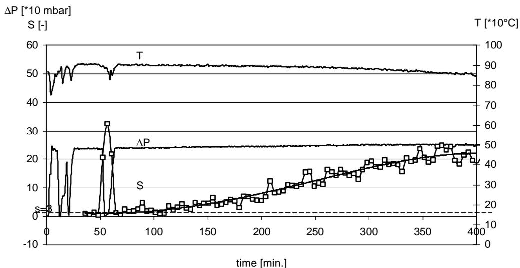
Figure 2.13 *The  $S$ -value measured during a seven hour test in which a 90/10 (m/m) mix of wood and an agglomeration-sensitive fuel was combusted in a bench-scale fluidised bed reactor. The biomass ash was allowed to accumulate.*
