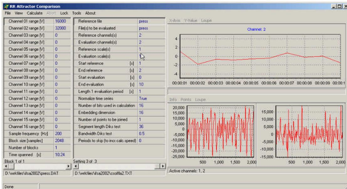
Figure 3.4 A screenshot of AttCom. On the left-hand side, the settings are given. The upper right panel gives the  $S$ -value as a function of time; the measured pressure signals are given in the right bottom corner.
