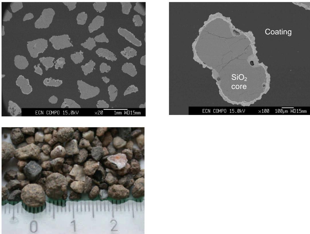
Figure 3.8 *SEM backscatter (top) and optical images (bottom) of 12.08.2002 bed material, collected before installation of the automated sieve. Most particles consist of a single (not-fragmented) SiO<sub>2</sub> core with an ash coating on the outside.*
