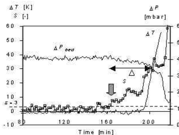
Figure 2.1 *The effectiveness of EARS is demonstrated in a bench-scale miscanthus gasification test at 760°C [3].*
