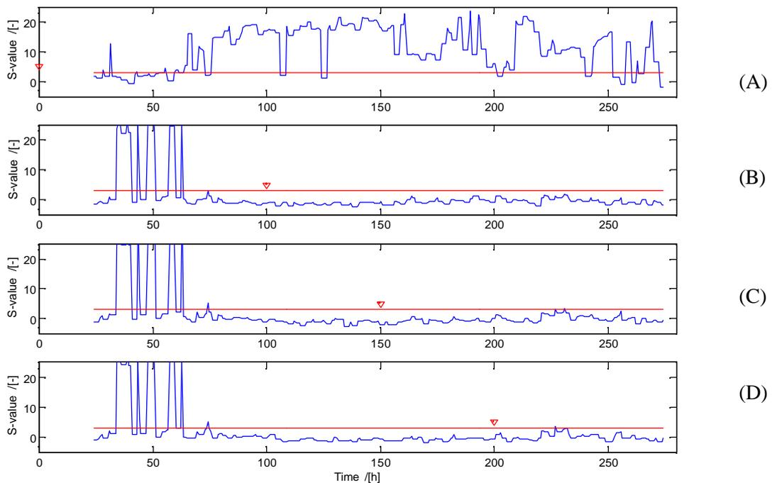
Figure 3.20 Results will be influenced by the location of the reference time period, indicated by  $\blacktriangledown$ . Situations A to D represent the effect of the location of the reference period on the filtered  $S$ -values during a test period in week 49. (A): the reference period is located in a different process operation regime. (B) to (D): the reference period is taken at various moments in the same and constant operation regime.
