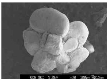
Figure 1.1 *Initial agglomerate of sand particles.*
