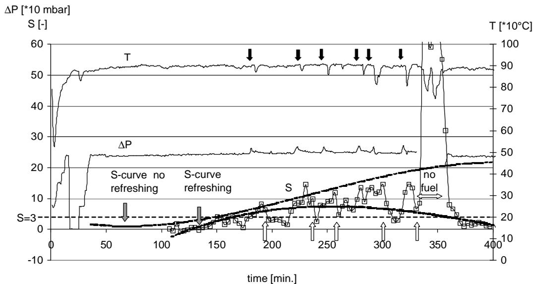
Figure 2.14 The  $S$ -value measured during a similar, seven hour combustion test. Periodically, a small part of the bed material was discharged and replaced by fresh (uncoated) sand. The black arrows indicate the replacement of bed material, while the open arrows indicate the reaction of the  $S$ -value.
