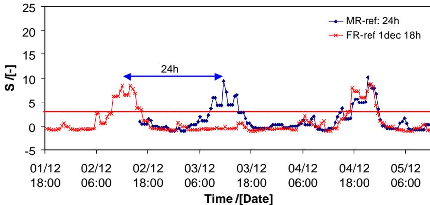
Figure 3.17 Example of the moving reference characteristic signalling a disturbance twice during the test period in week 49.2003 in the Essent 80 MW<sub>th</sub> BFB combustor.
