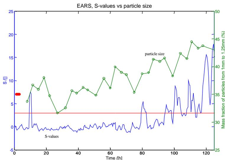
Figure 3.11 *The relation between the  $S$ -value measured at pressure probe position no.2 and the changes in particle size, measured by sieve analyses of the recycle stream in week 33.2002. The reference time period is symbolized by •.*
