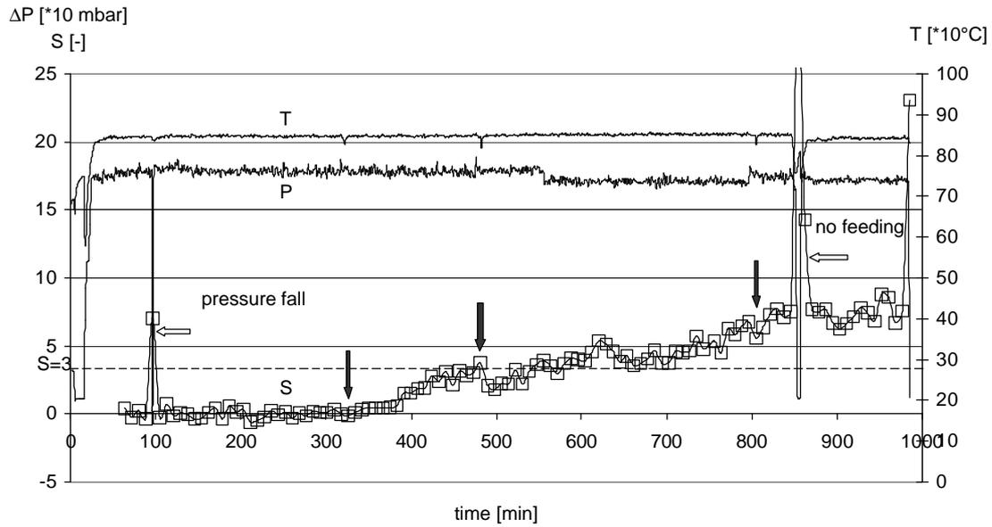
Figure 2.6 *Calculated S-value during wood combustion test at 850 °C and 5% excess oxygen. The black arrows indicate the replacement of bed material.*
