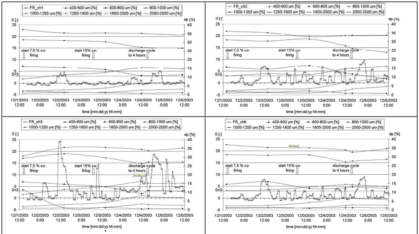
Figure 3.28 The  $S$ -values for pressure probe positions 1,2,3 and 6 during the test week, using a fixed reference (taken at 01.12.2003, time 16:00-16:20h). Included are the corresponding particle size distributions determined by sieve analysis.
