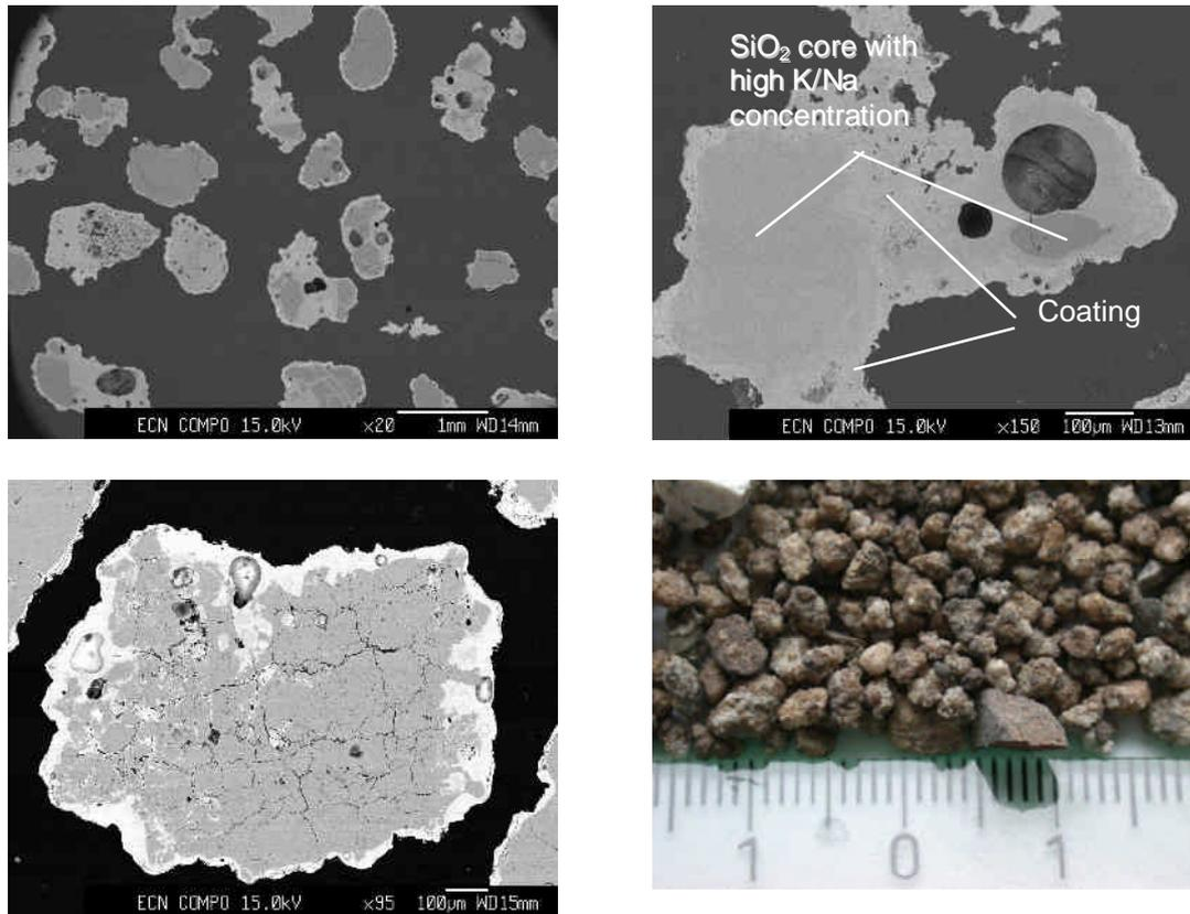
Figure 3.9 *SEM backscatter and optical images (bottom right) of 24.09.2002 bed material collected after installation of the automated sieve. Many particles consist of multiple SiO<sub>2</sub> core fragments with an ash coating between them and on the outside. The originally (pure) SiO<sub>2</sub> core particles are often ‘impregnated’ with significant amounts of K and Na. The bottom-left image shows many cracks inside the SiO<sub>2</sub> core particle.*
