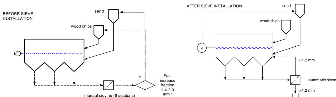
Figure 3.5 Fuel, fresh sand and bottom ash flows before (left) and after (right) installation of sieve at BEC power station.
