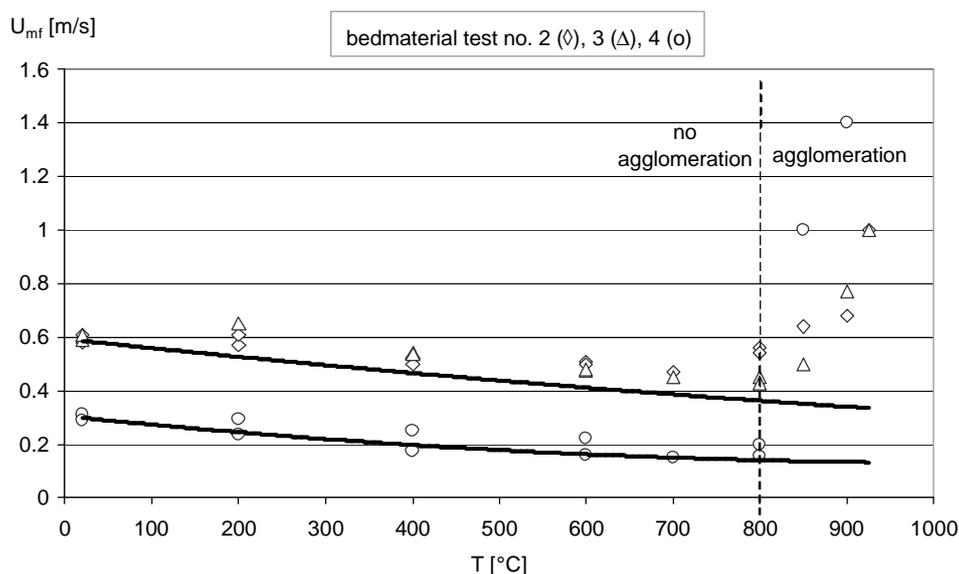
Figure 2.9 Minimum fluidising velocity determined as a function of temperature. The lines represent calculated values.
