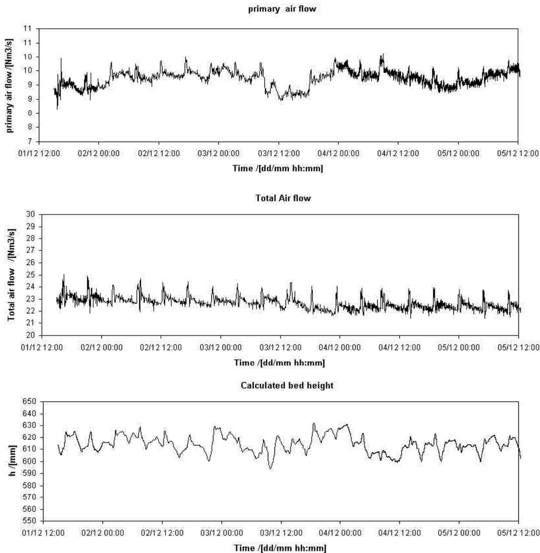
Figure 3.27 Relevant process data recorded during the test week.
