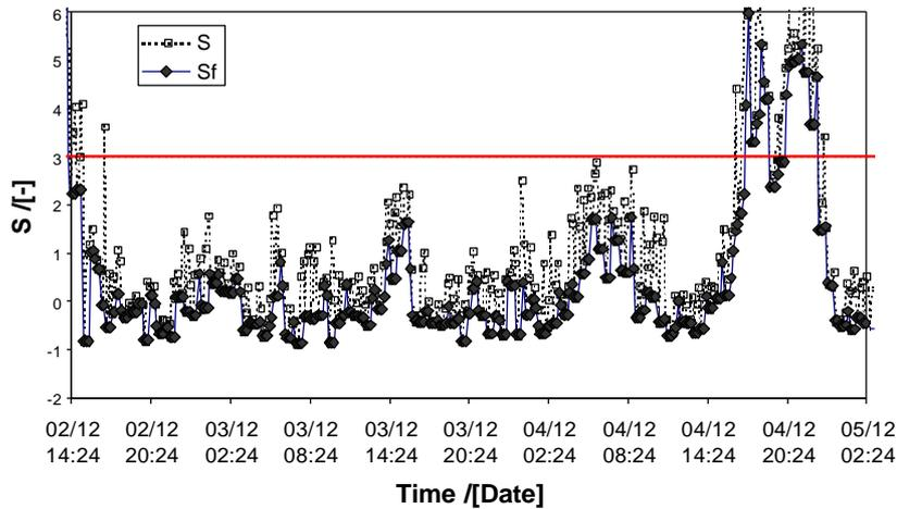
Figure 3.19 The effect of filtering illustrated during a monitored time series in the Essent combustor ( $S_f$  represents filtered values).
