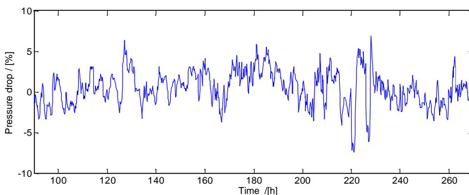
Figure 3.13 *The normalized deviation of the pressure drop over the fluidised bed.*
