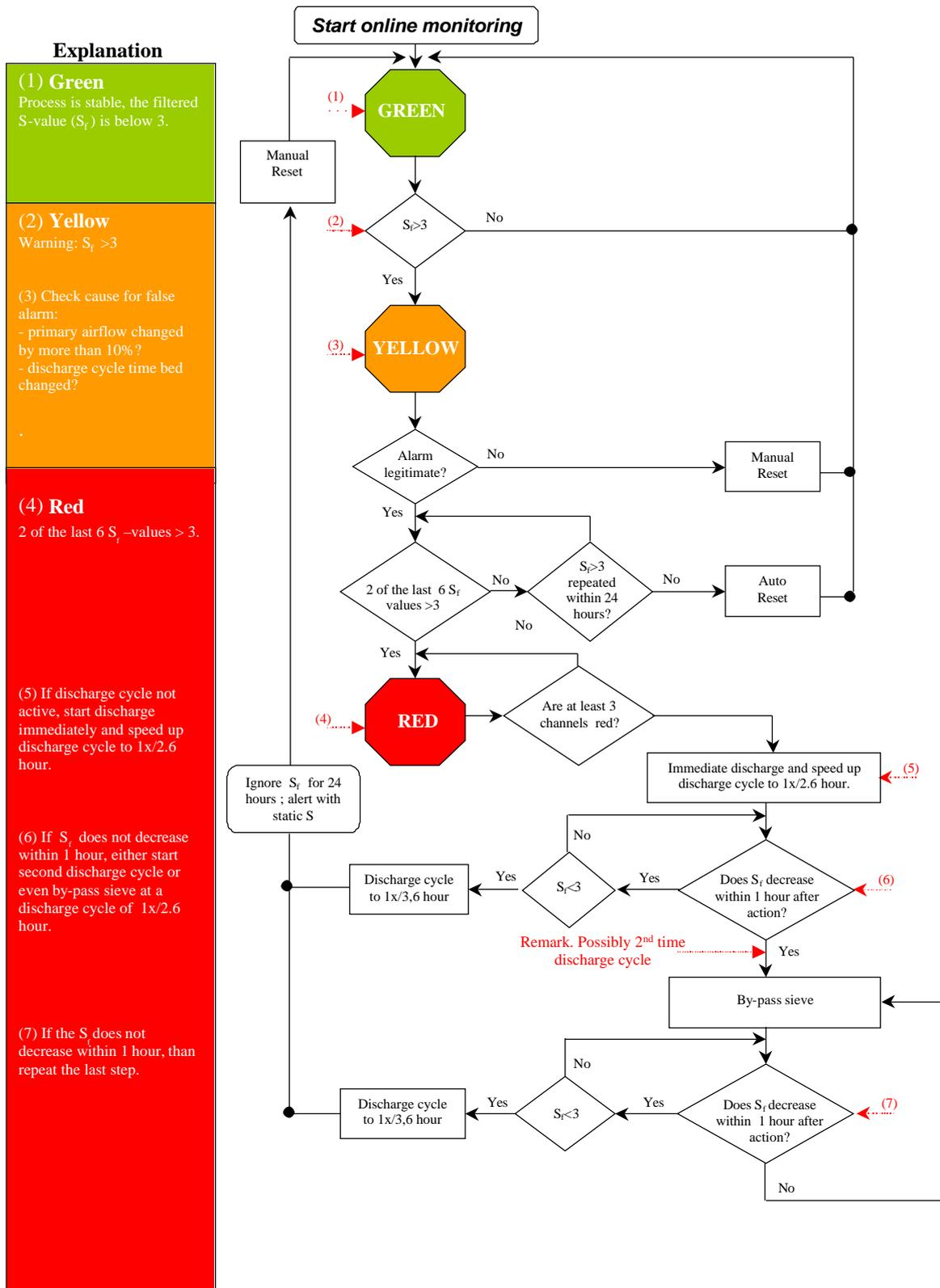
Figure 3.23 Instruction set for EARS-based agglomeration management controlling the rate of sand replacement in the Essent 80 MW<sub>th</sub> BFB combustor.
