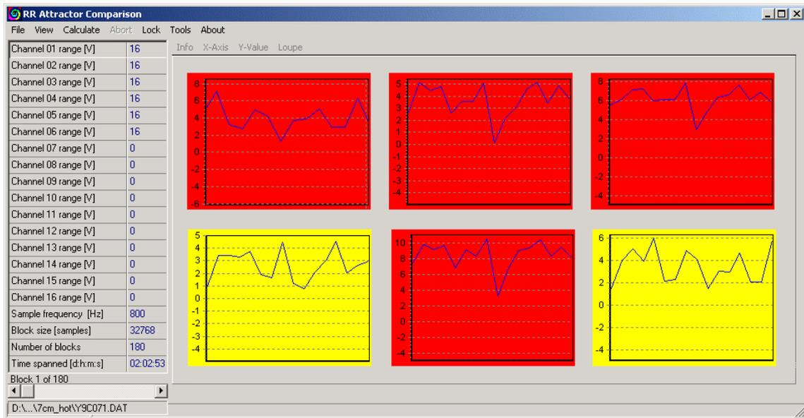
Figure 3.22 Screenshot of the EARS prototype for testing by the BFB operating staff. Top: all six bed sections normal; bottom: two bed sections give an agglomeration warning, four give an agglomeration alarm.
