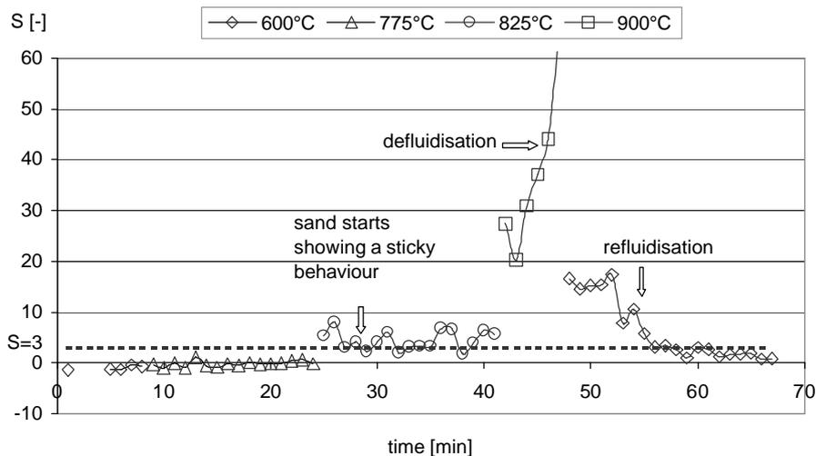
Figure 2.10 *The influence of particle stickiness on fluidisation behaviour, demonstrated by measuring the *S*-value of a fluidised bed of ash-coated (spent) particles at typical coating melt temperatures (see also Figure 2.9).*
