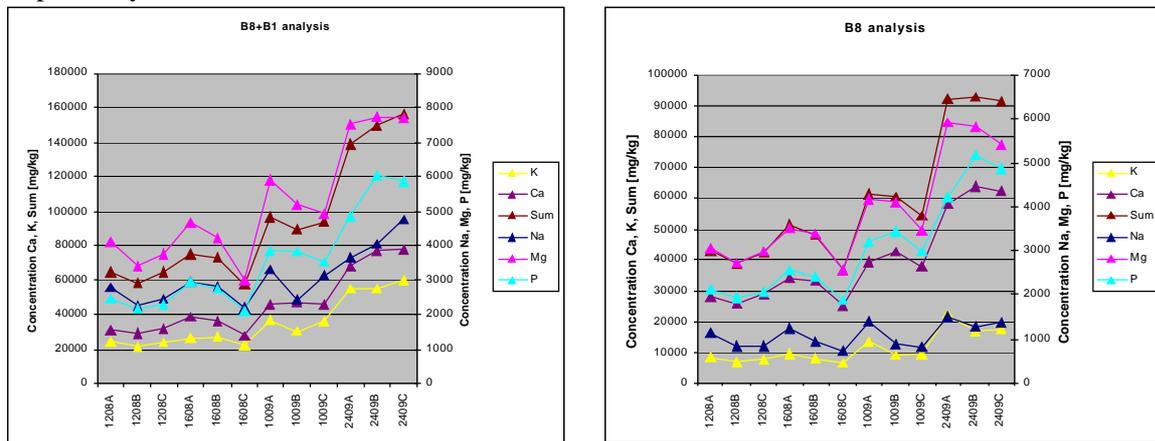
Figure 3.7 Chemical composition of bed material samples collected before (1208 and 1608) and after (1309 and 2409) installation of the sieve. A, B and C refer to size fractions 500-710, 710-1000 and 1000-1180  $\mu\text{m}$  respectively. The left figure gives the whole particle composition, while the right figure gives the composition of predominantly the outer particle layer (first, partial digestion).
