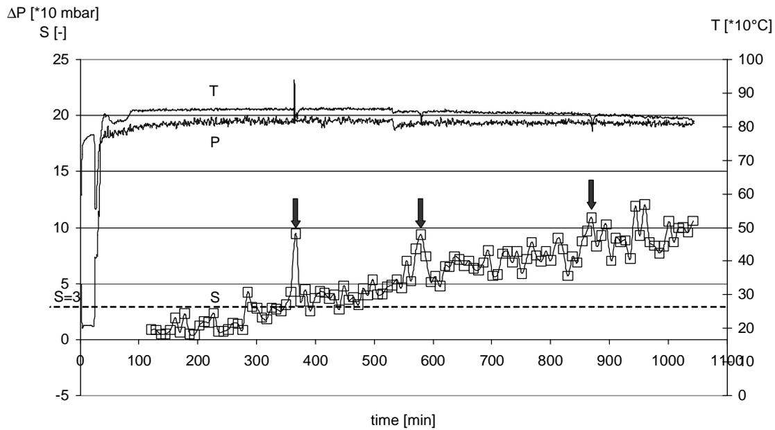
Figure 2.7 *Calculated S-value during wood combustion test at 850°C and 1% excess oxygen. The black arrows indicate the replacement of bed material.*
