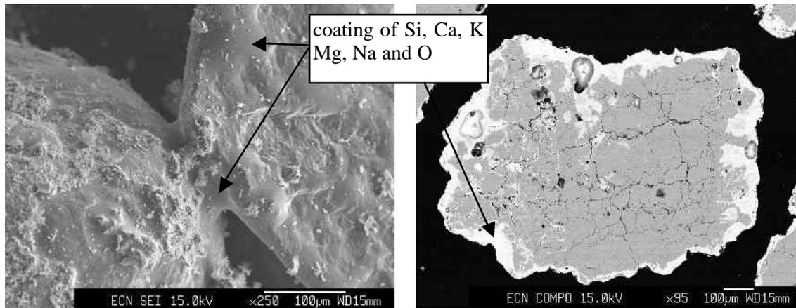
Figure 2.8 SEM micrographs of bed particles showing biomass ash-derived coating (left and right) and internal cracks (right). The left micrograph was obtained from test no. 2, the right was obtained from spent bed material.
