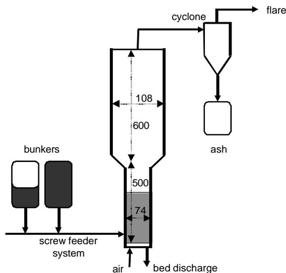
Figure 2.5 Schematic representation of the 1 kg/h bubbling-fluidised-bed gasifier/ combustor, sizes in mm.
