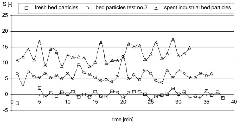
Figure 2.11  $S$ -values measured with different bed materials having the same particle size distribution and density but different particle sphericity.
