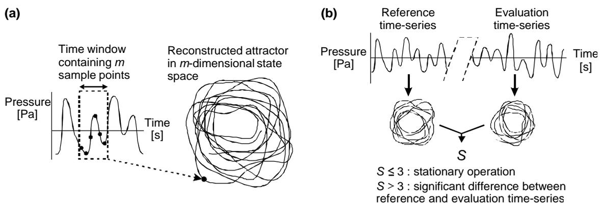
Figure 1.3 Schematic representation of (a) the reconstruction of an attractor from a pressure fluctuation signal, and (b) the comparison of attractors by the monitoring method.
