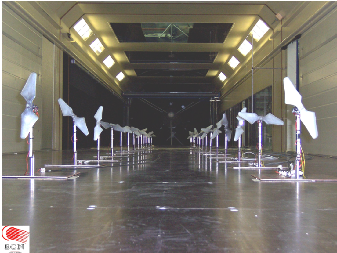
Figure 15: A farm of 14 rows of 2 model turbines on scale 1:400 in the boundary layer wind tunnel
