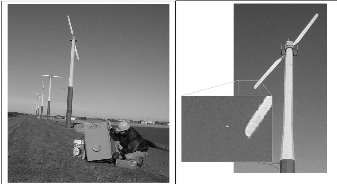
Figure 2.5: *On the left: Tennis ball machine used to simulate Birds (sparrow). On the right: tennis ball hitting the rotor of the wind turbine.*
