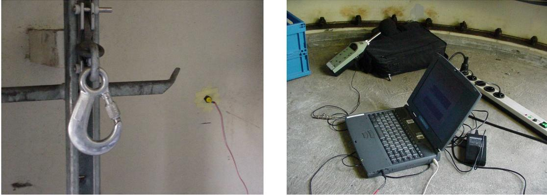
Figure 2.3: *On the left the microphone set-up is shown applying a microphone to the turbine wall (seen on the right in the picture). On the right the spherical sound registration inside the turbine tower is shown.*
