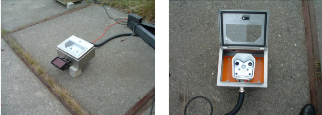
Figure 4.5: Camera housing used for night tests with the IR light source mounted on top
