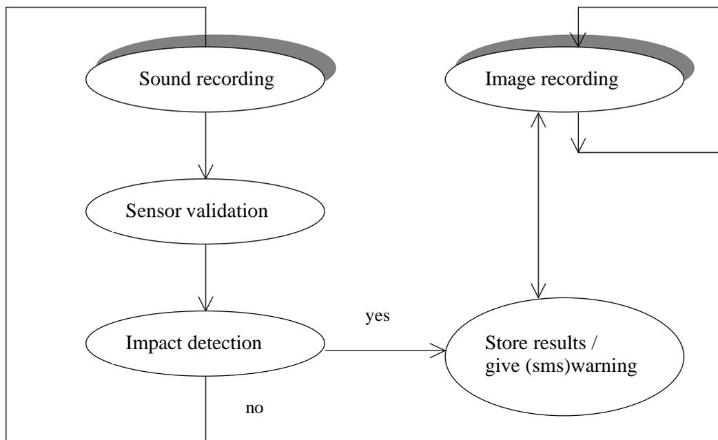
Figure 5.1: *Principle of the WT-Bird software*
