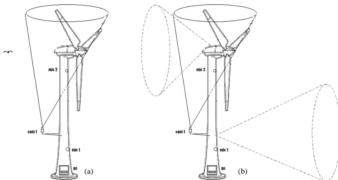
Figure 6.1: *Different possibilities for placing microphones and cameras*
