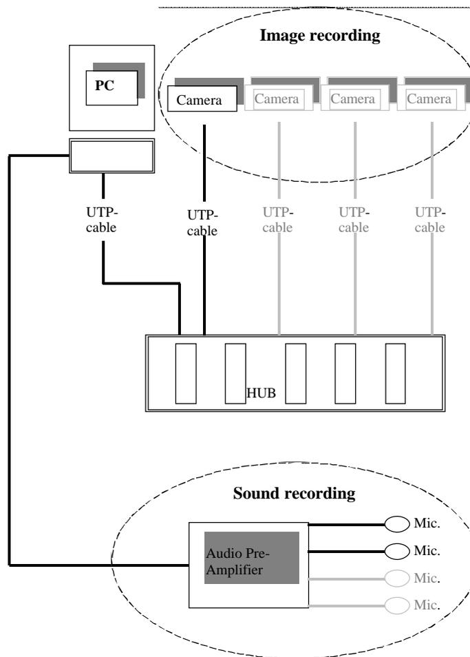
Figure 6.2: Schematic overview of the modular network configuration
