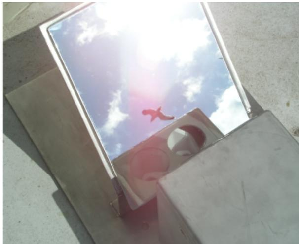
Figure 6.4: *Camera housing with mirror*
