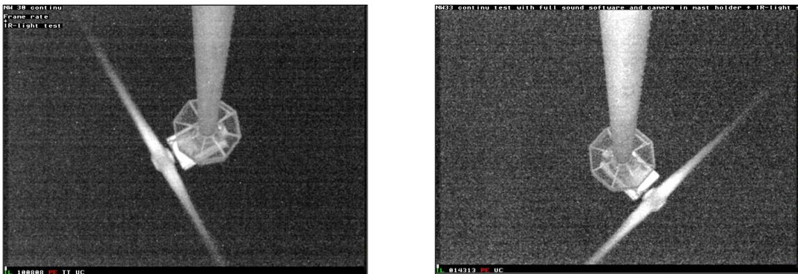
Figure 4.6: Test with external IR source, left without additional housing, right with additional housing.
