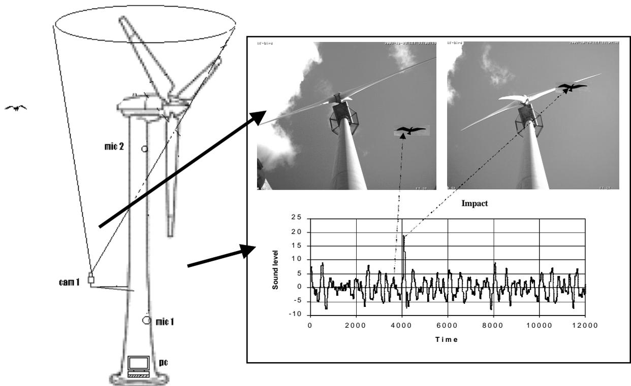
Figure 2.1: Principle of operation of the bird collision recorder
