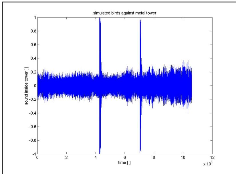
Figure 2.4: *Sound registration with two sand bags against the mast (LW18/80 "Anna Paulowna"). The hits are recognised by the two events with high amplitudes of the sound recording.*
