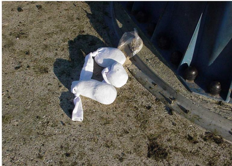
Figure 2.2: *Examples of the sand bags that were used to mimic birds colliding with the mast of the turbine.*
