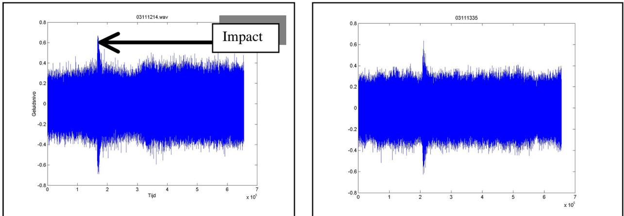
Figure 2.6: (On the left) Impact of a tennis ball against the rotating rotor blade (WP "Slag Dobbelsteen"). (On the right) Impact of a tennis ball against rotor blade and mast.
