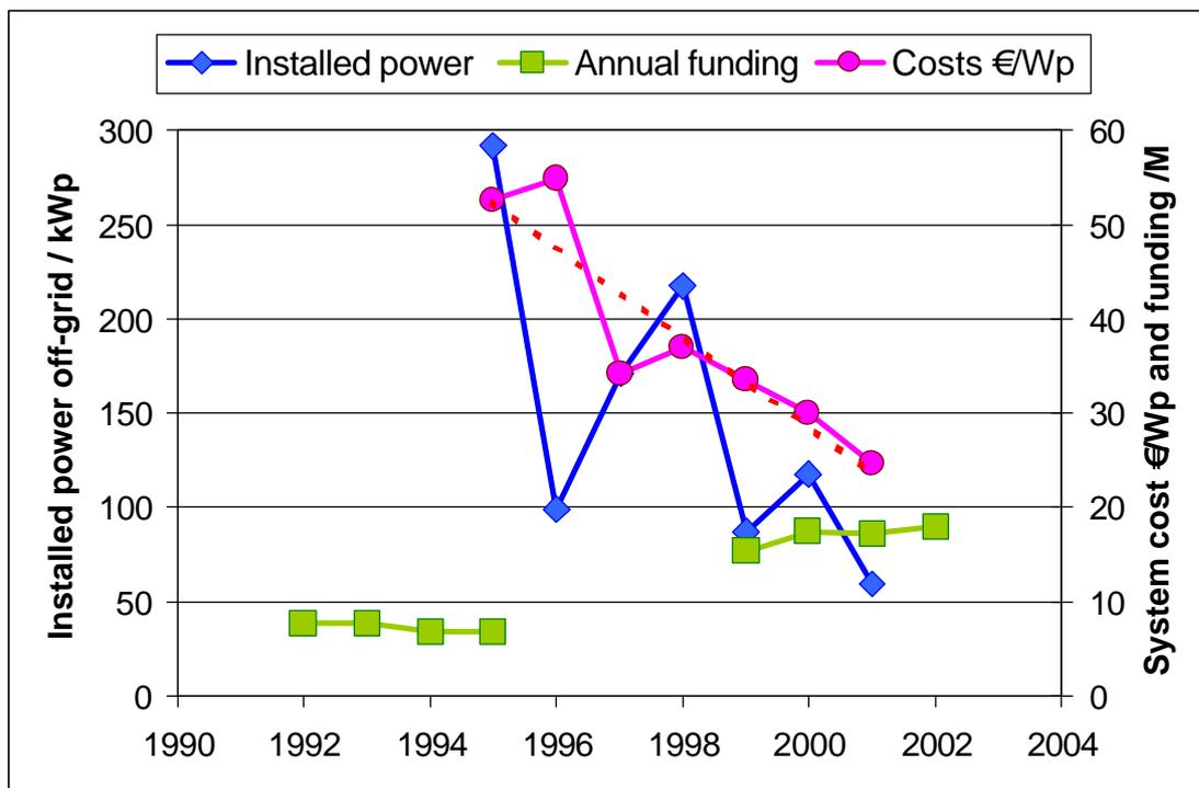
Figure 4.12 Average systems price for off-grid applications and installed power
