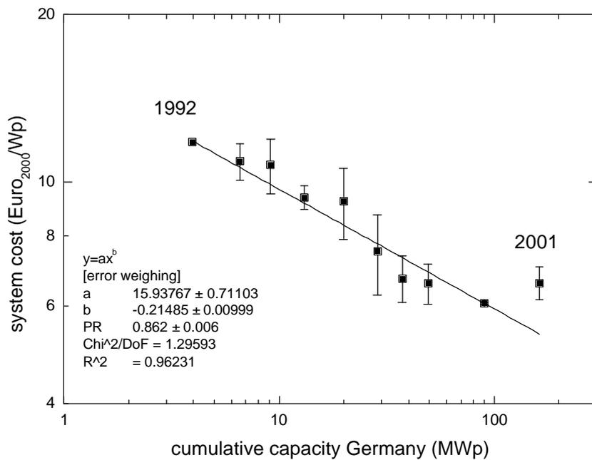
Figure 3.4 *Experience curve for total system prices in Germany, using installed capacity in Germany for x-axis. The analysis of this compound system price gives erroneous results because modules learned on the global market that had a much slower growth than the German market over that period*
