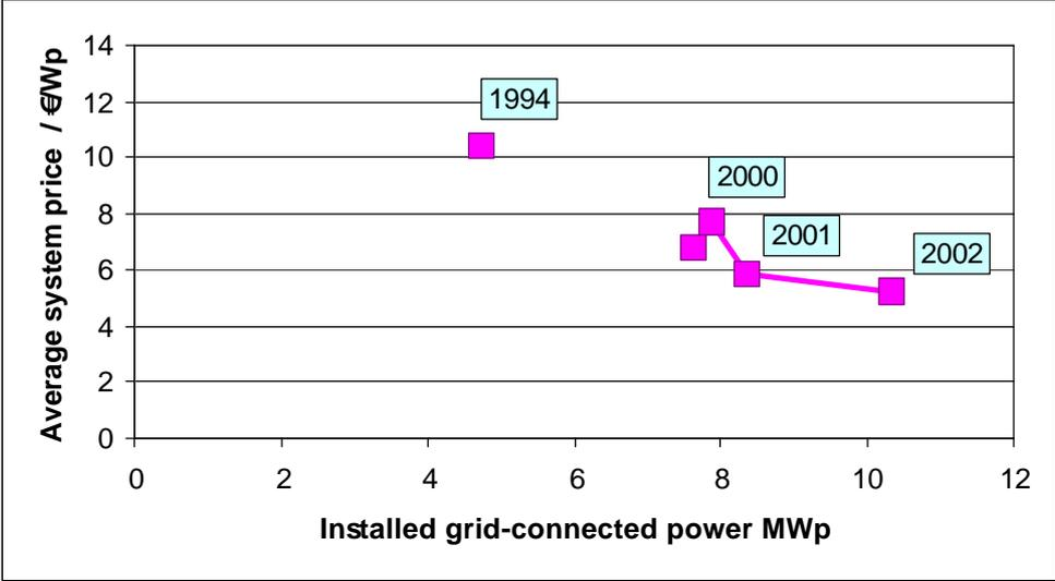
Figure 4.17 Experience curve for grid-connected PV in Italy
