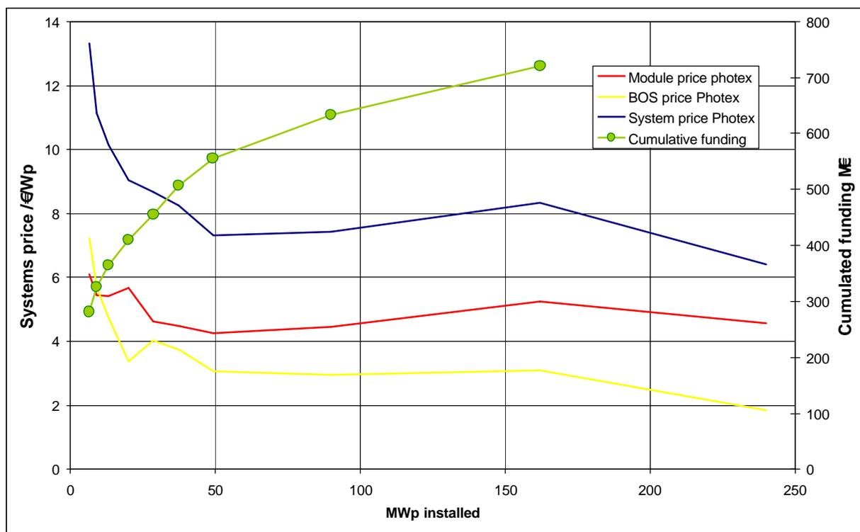
Figure 4.10 Total cumulated funding and average system price over cumulated installed power from 1993 to 2002
