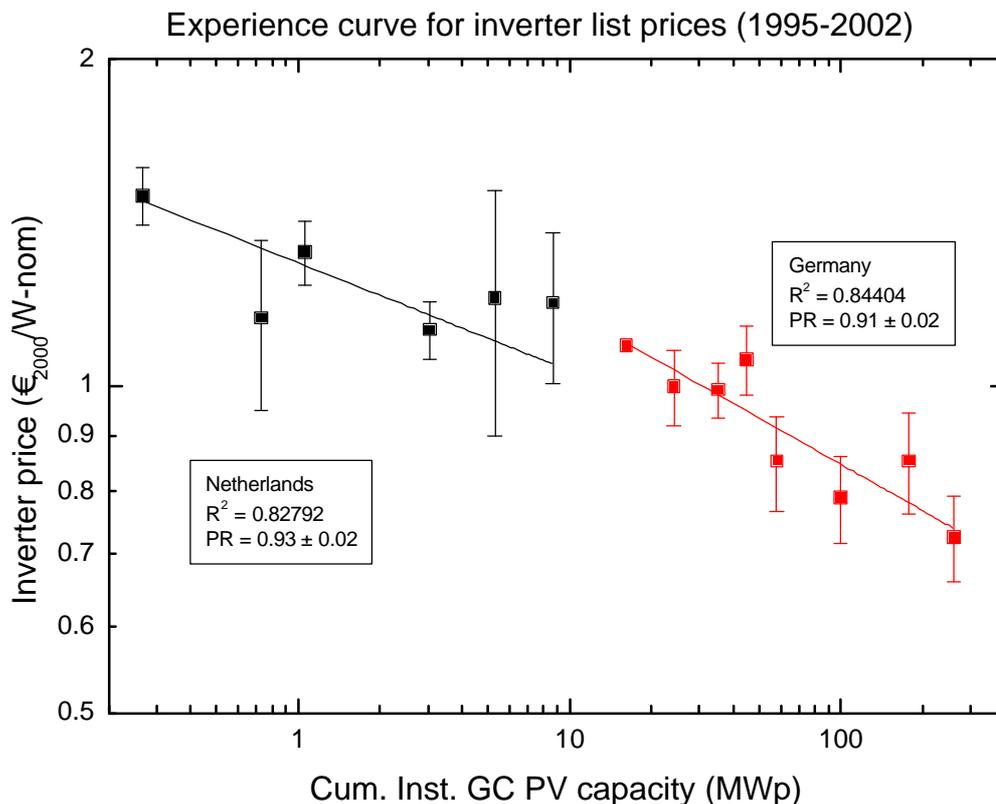
Figure 3.12 Experience curve for inverters in Germany and the Netherlands. Price data were derived from manufacturer catalogues, for the x-axis parameter the cumulative capacity (source IEA) of grid-connected PV systems in each country was used.
