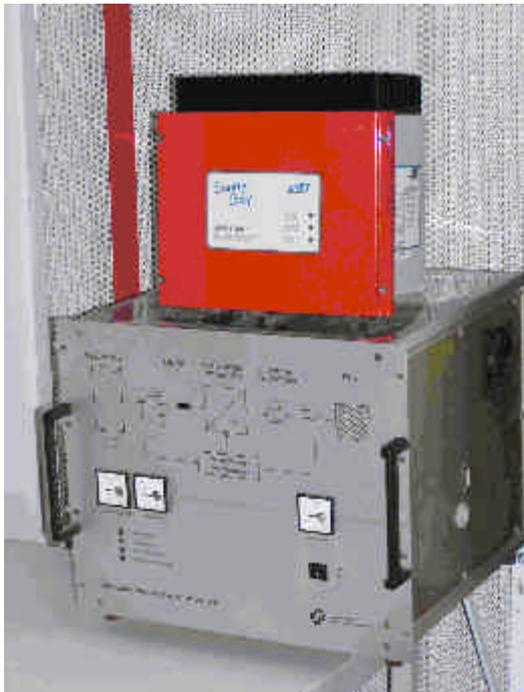
Figure 5.8 A 1,5 kW inverter from 1989 (bottom) and a modern 1.1 kW inverter (top) with far more functionalities
