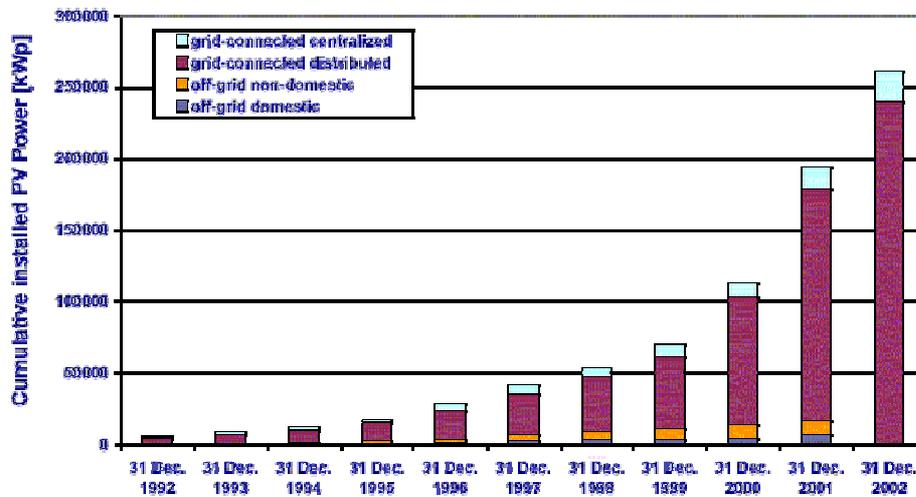
Figure 4.7 *Installed power in Germany (Source IEA)*
