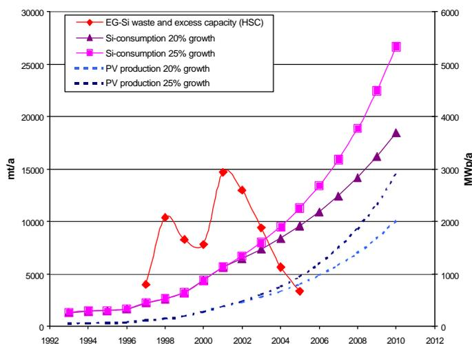
Figure 5.5 Supply and consumption of high-purity silicon (EG-Si) for the PV industry
