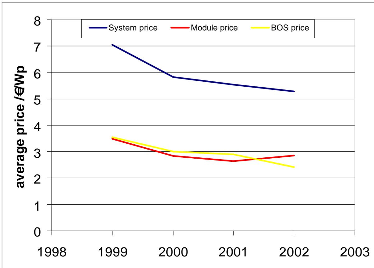
Figure 4.14 Price evolution curve for grid-connected PV in France
