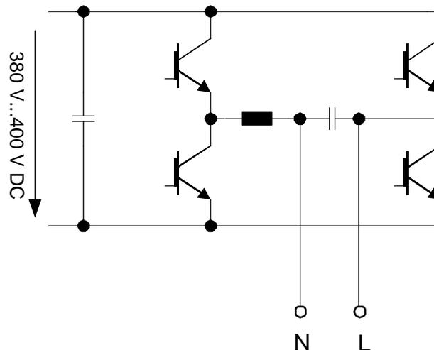
Figure 5.9 An “H-Bridge” which is a typical part of an inverter without galvanic separation or with a high frequency (> 10 kHz) DC/DC-Transformer
