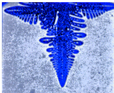
Figure 2-23: Dendritic growth as a result of 2-dimensional solidification of a metal. The finger-like shape of the solid results from instantaneous freezing of metal atoms at the growth surface, upon arriving from the melt.
