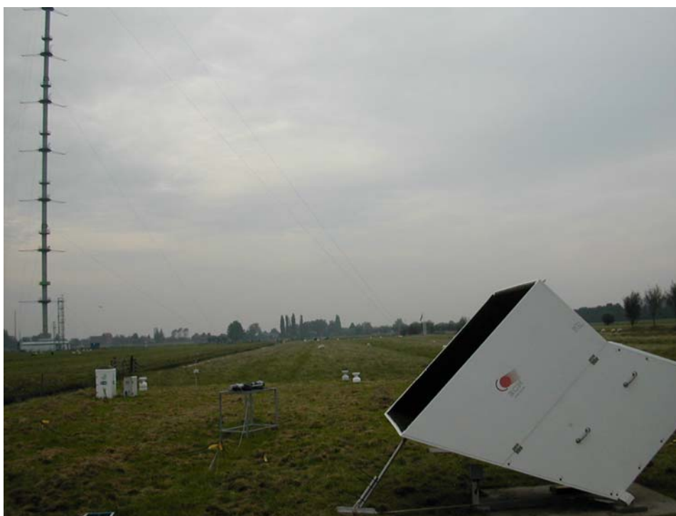
Figure 1: SODAR tilted towards 250 degrees
