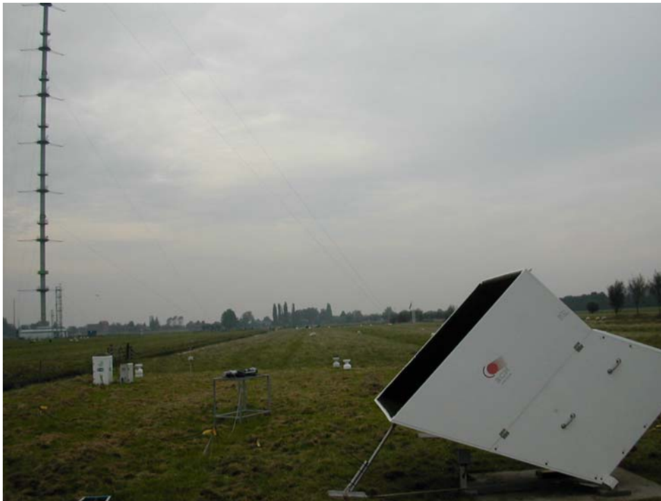
Figure 4: SODAR tilted towards 250 degrees
