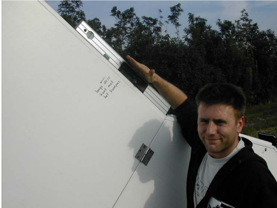
Figure 7: A measurement of the tilting angle is taken with the digital level.
