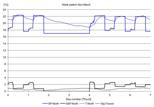
Figure 10.6 Setpoints and temperature for north-segment. The lower lines indicate the sigma of averaging
