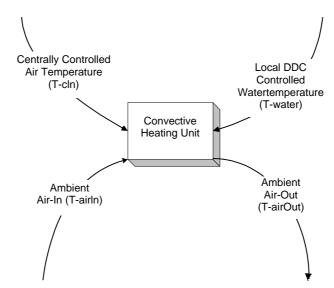
Figure 10.2 Convective heater model
