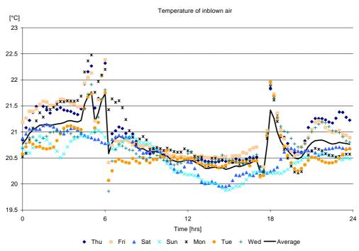
Figure 10.8 Temperature of in-blown air
