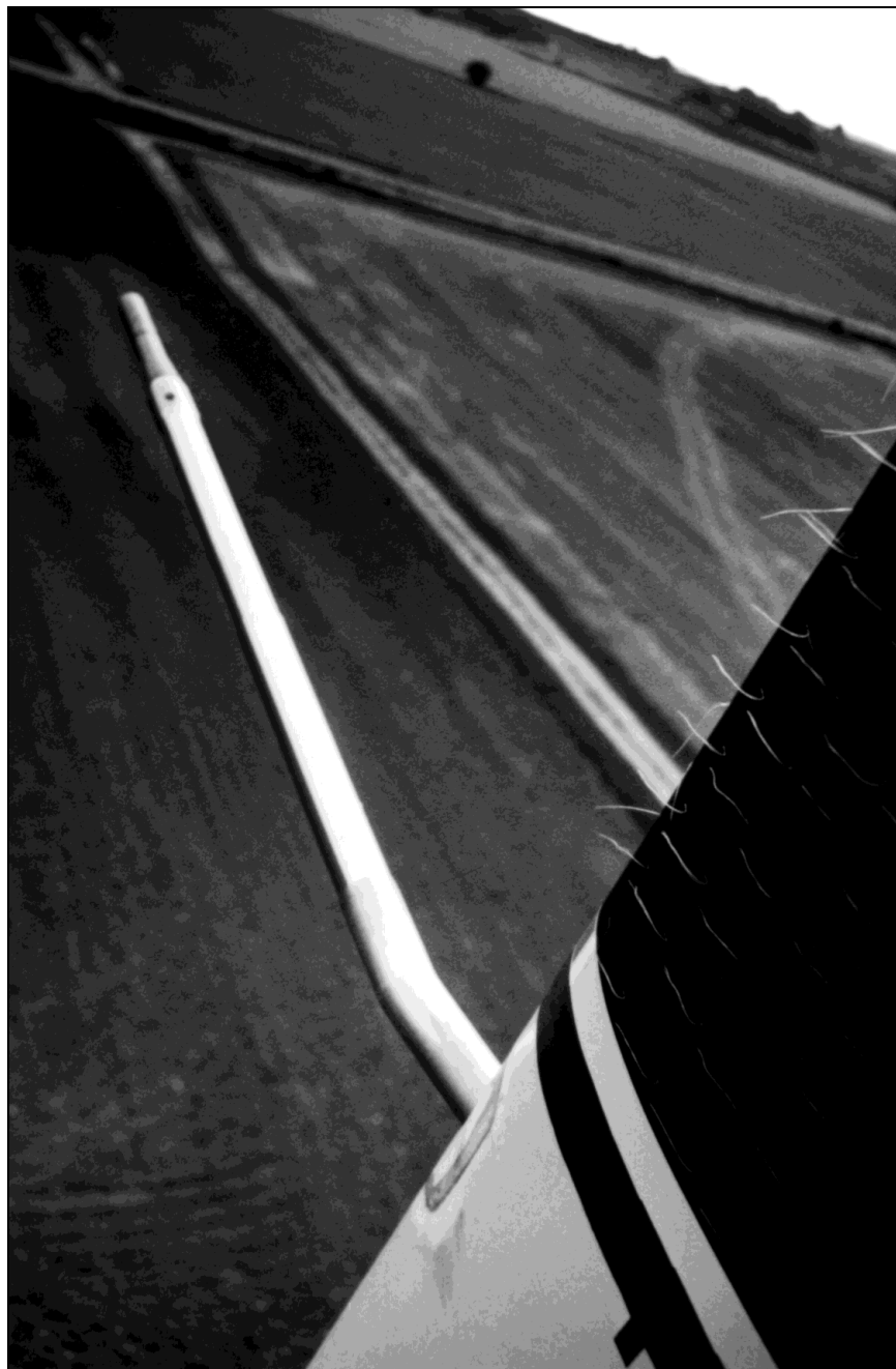
Figure 5.30 RISØ , The five hole pitot tube measuring the inflow velocity vector to the blade
