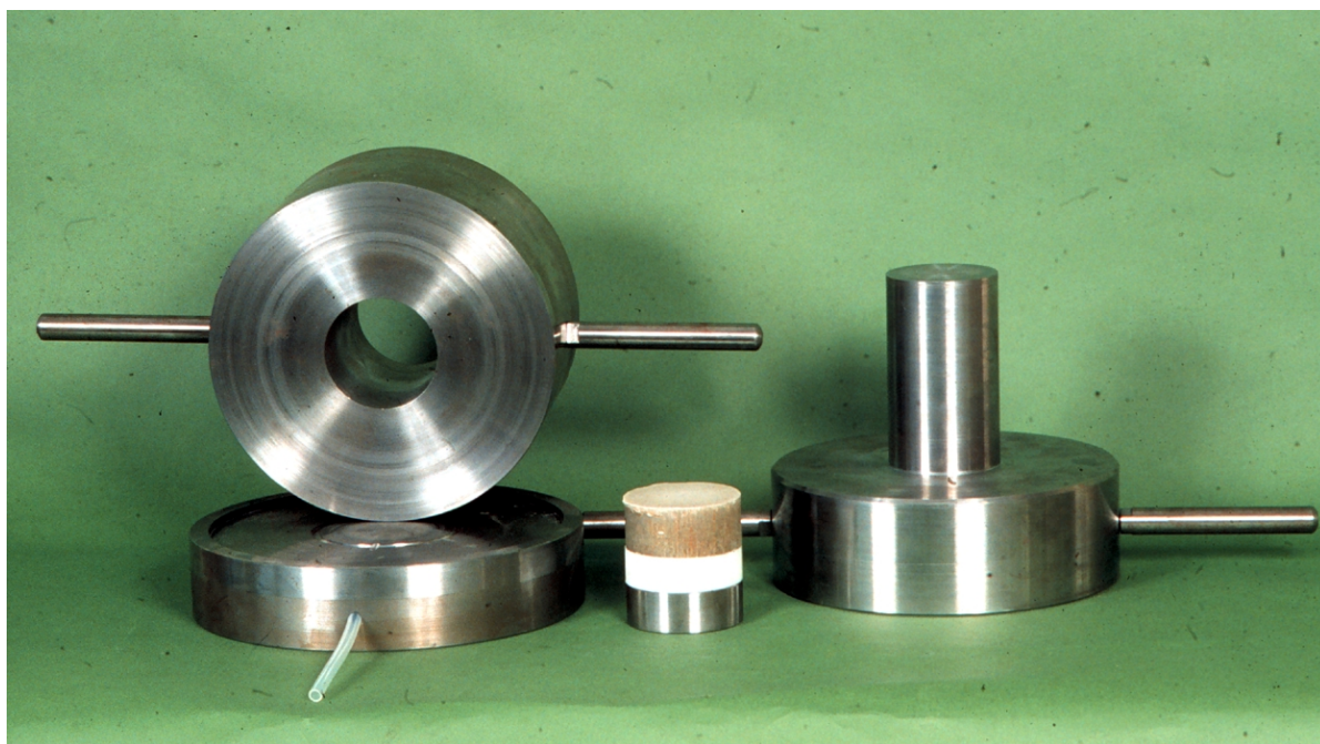
Figure A3.1: Apparatus for expression of pore water.
