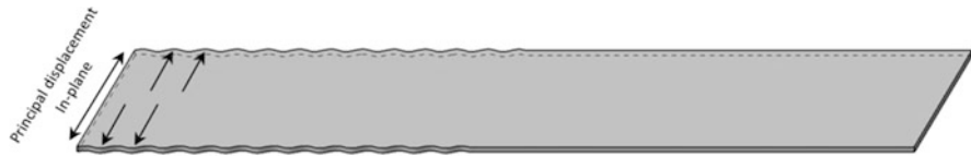
Fig. 3.10 Shear mode of propagation
