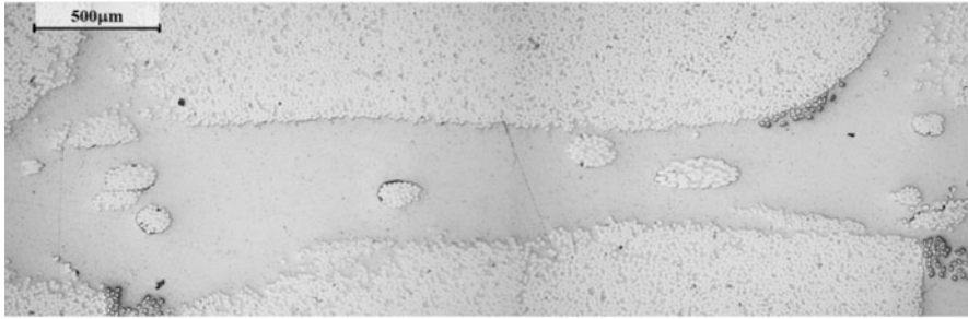
Fig. 23.5 Microstructure of a unidirectional composite from the load carrying beam
