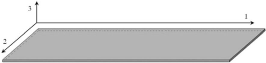
Fig. 3.7 Coordinates for thin plate-like structure
