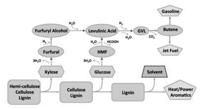
Figure 9.10 Roadmap for conversion of lignocellulosic biomass (rectangles) to chemicals (ovals) and fuels (pentagons), passing through the intermediate formation of C<sub>5</sub> and C<sub>6</sub> sugars (hexagons). Dashed arrows indicate processes that can be carried out using a lignin-derived organic solvent for the production of furfural, HMF, levulinic acid, and GVL [50].
