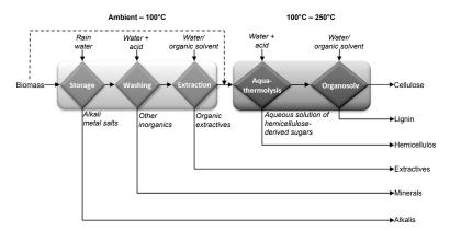
**Figure 9.2** Staged solvolysis of lignocellulosic biomass for primary fractions.
