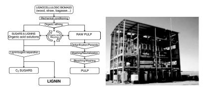
**Figure 9.5** Process scheme and photograph of the CIMV organic acid-based organosoly process [33].
