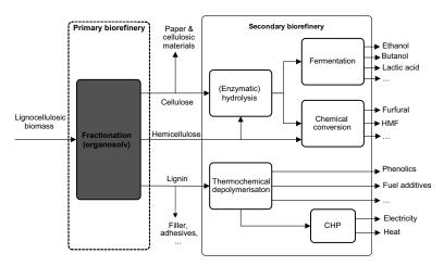
**Figure 9.7** General layout of an organosolv-based biorefinery [30].
