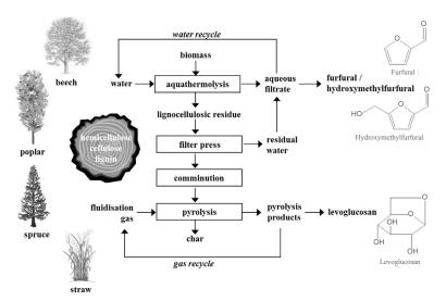
**Figure 9.3** Hybrid biorefinery concept [1].
