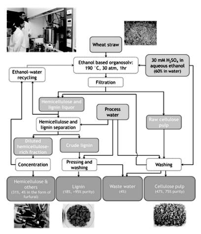
Figure 9.4 Fractionation of wheat straw by aqueous ethanol organosolv [31].
