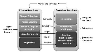
Two-step biorefinery concept featuring staged solvolysis in the Figure 9.1 primary biorefinery and dedicated processing in the secondary biorefinery. See also Color Insert.
