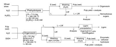
Figure 9.9 Experimental approach of direct organosolv vs. prehydrolysis—organosolv of wheat straw. Reprinted from Ref. [27], Copyright 2012, with permission from Elsevier.
