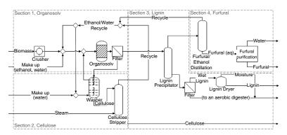
**Figure 9.8** Ethanol-based organosolv biorefinery [34].
