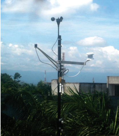
Wind and solar sensors on top of the roof of the Engineering faculty of USU, March 2011
