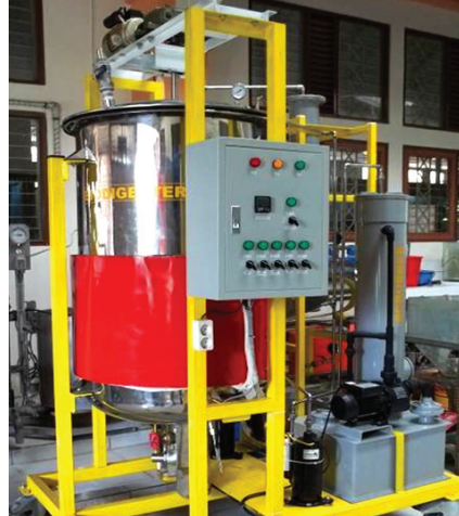
Biogas analysis and improvement system installed at UNDIP, October 2011
