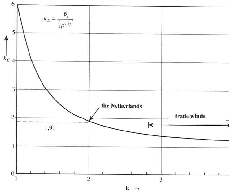
Fig. 2. The energy pattern factor  $k_E$  as a function of the Weibull shape parameter  $k$ .<sup>4</sup>
