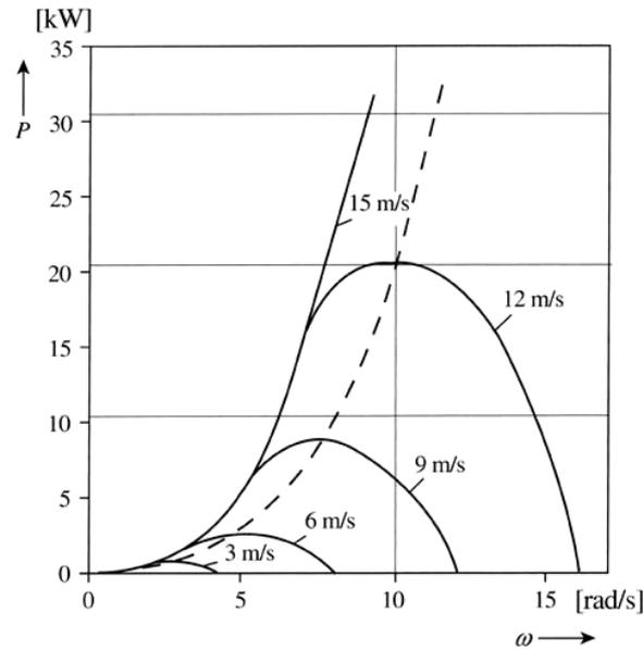
Fig. 9. Power characteristics of a rotor for various constant wind speeds. ( $P$  = power output at the rotor shaft,  $\omega$  = rotational speed of the rotor shaft. The dotted curve ( $P \sim \omega^3$ ) indicates the point of maximum efficiency for various wind speeds.<sup>4</sup>
