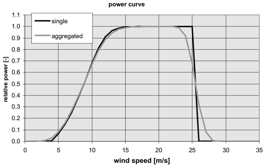
Fig. 20. Regionally averaged and single turbine power curve. The relative power is the power as normalized to the rated power.
