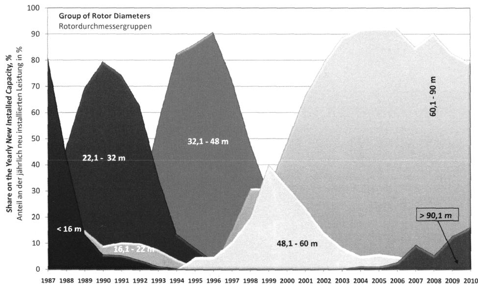
Fig. 23. Product cycles of commercial wind turbines based on rotor diameters.<sup>55</sup>
