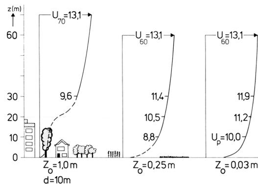
Fig. 5. Vertical wind shear for various values of the terrain roughness  $z_0$  for the same value of the meso wind speed  $U_m = 13.1$  m/s.<sup>7</sup>
