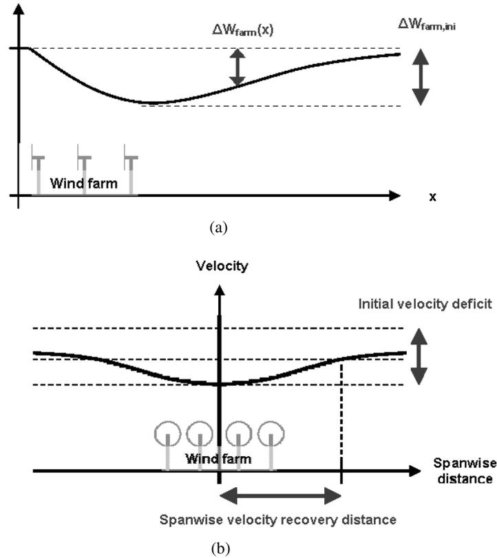
Fig. 19. Recovery of the velocity wake behind (a) and besides (b) a wind farm.<sup>32</sup>
