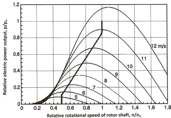
Fig. 13. Power-rotational speed curves of the wind turbine rotor and the electric generator load. From the points where both curves cross, the power-wind speed curve of a wind turbine can be constructed (see Fig. 15).<sup>19</sup>
