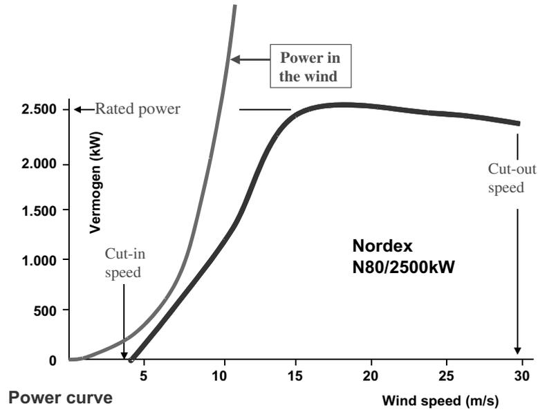
Fig. 14. Power–wind-speed curve as provided by the wind turbine manufacturer. These curves are being established according to standardized methods by independent testing stations.
