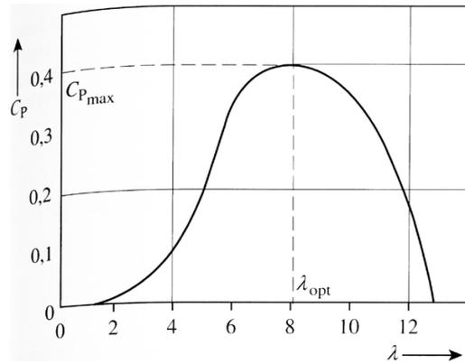
Fig. 10. The  $C_p - \lambda$  curve of a rotor with an optimum tip-speed ratio of 8.<sup>4</sup>
