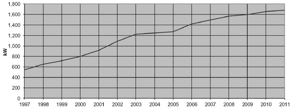
Fig. 24. Global average installed power per wind turbine within one year.<sup>52</sup>
