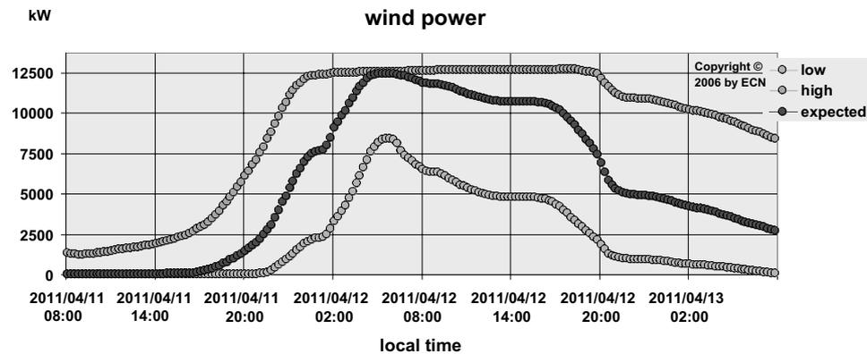
Fig. 21. Typical wind power forecast, consisting of the expected value and the confidence interval of the wind power. This forecast is valid for a wind farm with a nominal power of 12.5 MW and a turbine hub height of 70 m.
