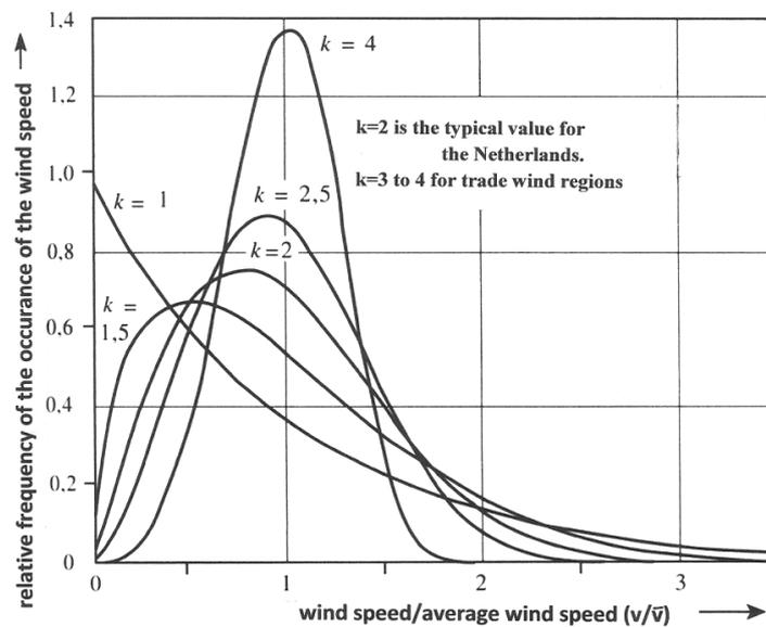
Fig. 1. Weibull distributions for various values of the shape factor  $k$ :  $k = 4$  is a typical value for the trading winds,  $k = 2$  is typical for moderate coastal areas e.g. in North Western Europe, and  $k = 1$  for polar areas.<sup>4</sup>
