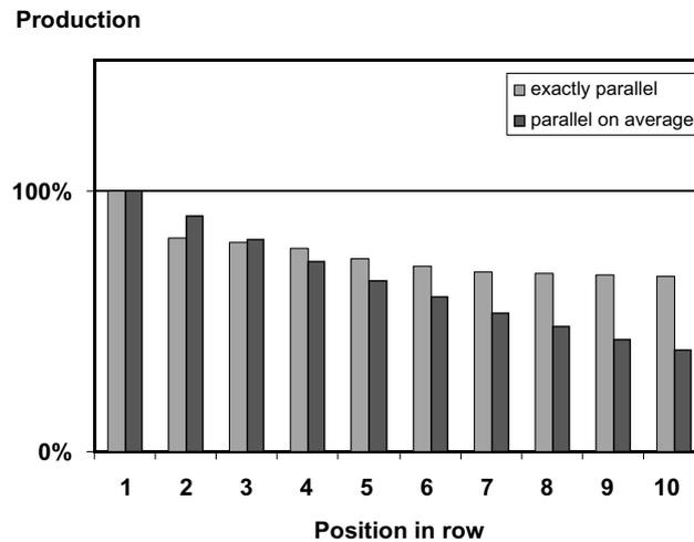
Fig. 18. Production along a row of wind turbines if the wind is blowing (a) exactly parallel to the row and (b) parallel to the row on average only.
