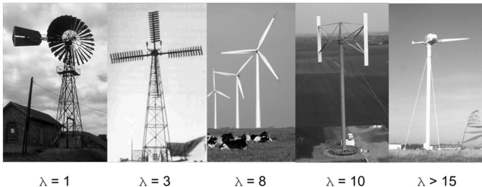
Fig. 11. Various types of rotors. On the left a slow-running wind pump. The other wind turbines are electricity-producing machines with increasing tip speed ratio. Three-bladed machines are the most applied ones because of the tradeoff between dynamic mechanical loading and rotational speed of the main shaft. Photographs 1,3,4 and (from left to right): Jos Beurskens.
