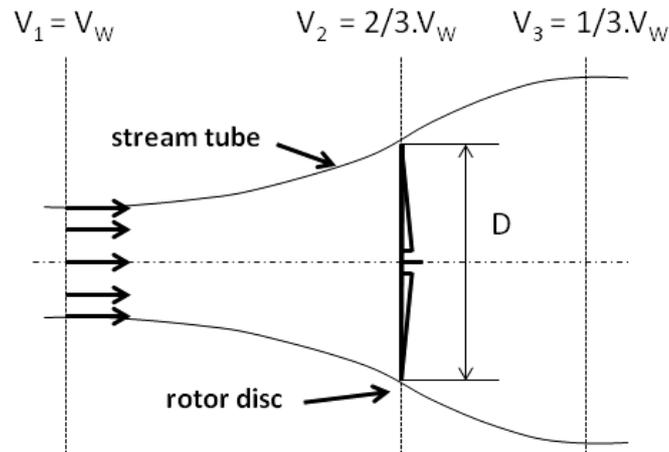
Fig. 8. The flow tube of a wind turbine rotor, explaining the momentum flow theory. The volume behind the rotor is called the wake.
