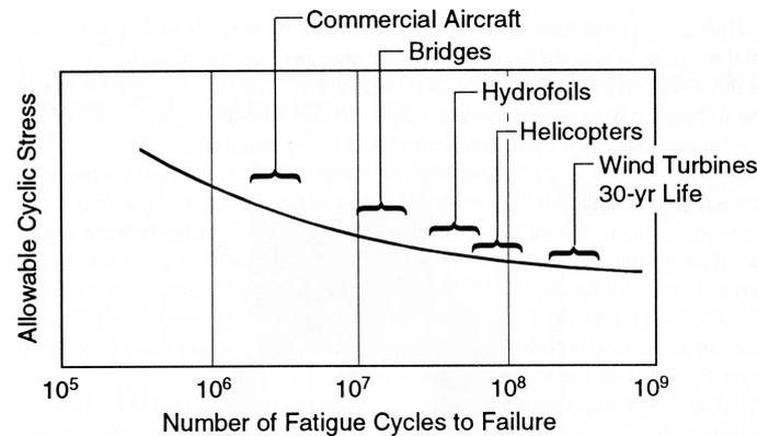
Fig. 16. Fatigue loading of a wind turbine compared with other structures and machines.<sup>25</sup>
