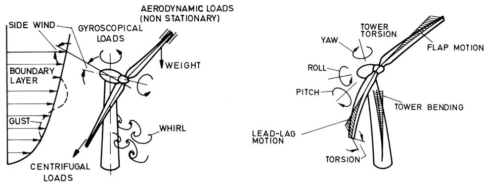
Fig. 15. Mechanical excitations and responses of a wind turbine structure.
