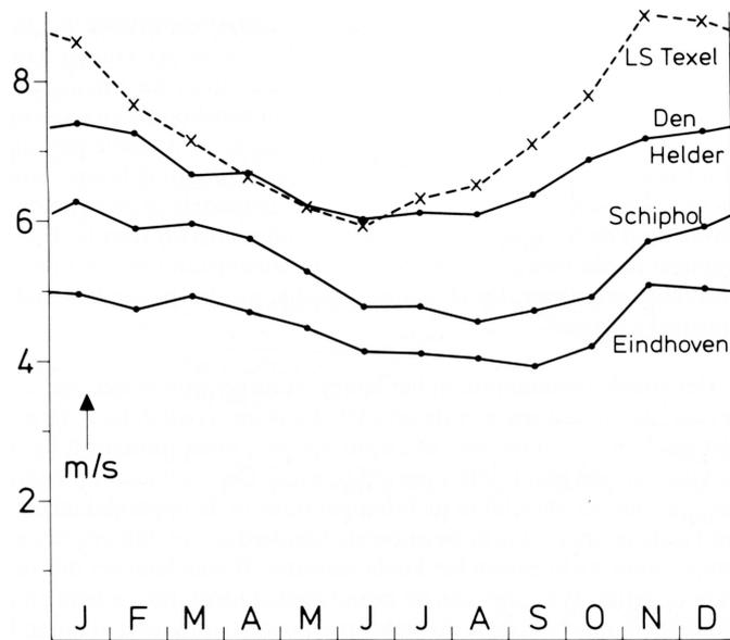
Fig. 4. Average monthly change of the wind speed at four metrological stations in the Netherlands.<sup>7</sup>
