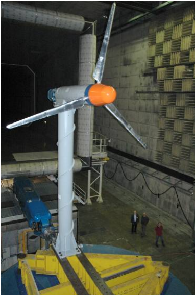
Figure 9-3: The Mexico wind tunnel experiment in the DNW wind tunnel. Source: [ECN, photo Toon Westra]
