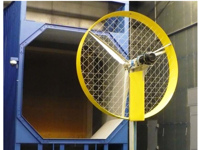
Figure 9-9: The rotor of the wind race car of ECN in the OJF [Source ECN, Picture by P. Eecen]
