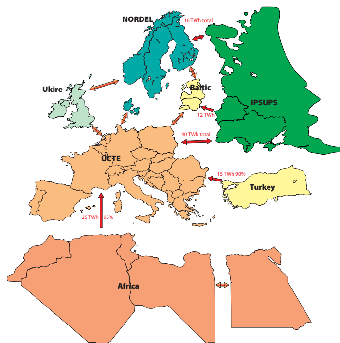
Figure 3.2 Synthesis of the electricity exchanges (volumes, directions and percentage utilization 2030, reference scenario)
