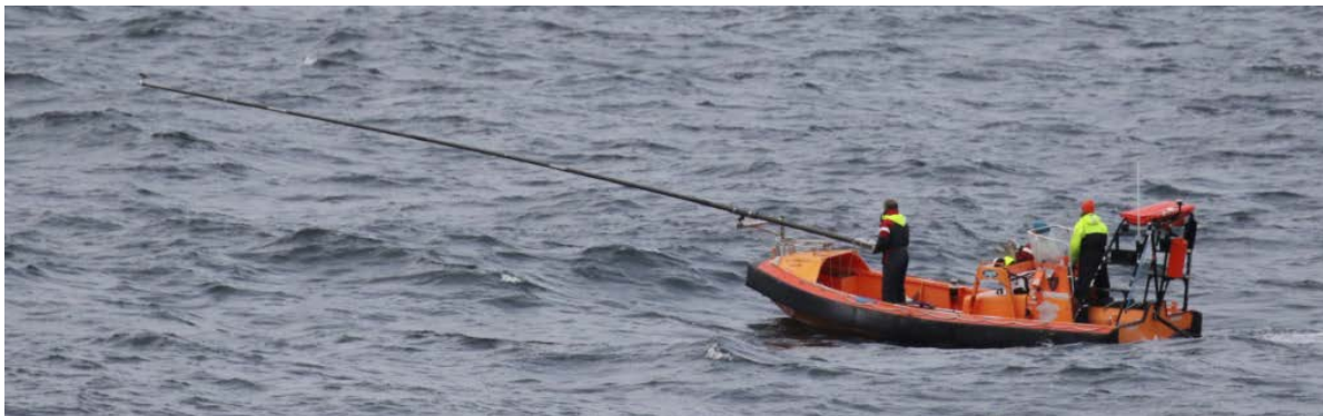
Tag Boat 2 (TB2) will be the main platform. It will be equipped with a swivel in the bow for the cantilever pole.
