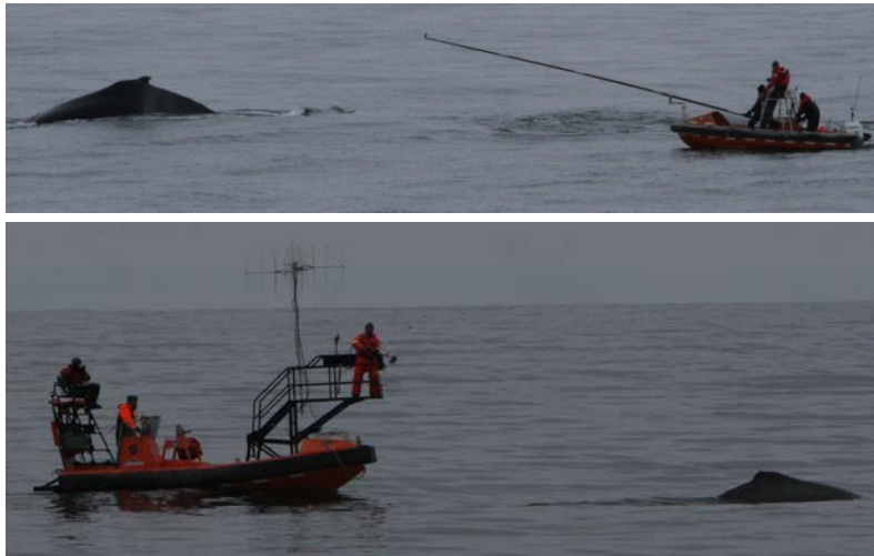
Tag Boat 1 (top) and Tag Boat 2 (bottom). TB1 will be equipped with a swivel in the bow for the cantilever pole. TB2 can be installed with a 2 person elevated MMO-station behind the driver for tracking whales, and an elevated shooting platform in the bow for the tagging.
