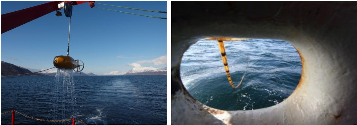
The sonar source SOCRATES (left) and acoustic array Delphinus (right) safely recovered on the Sverdrup during a previous trial (3S-12).
