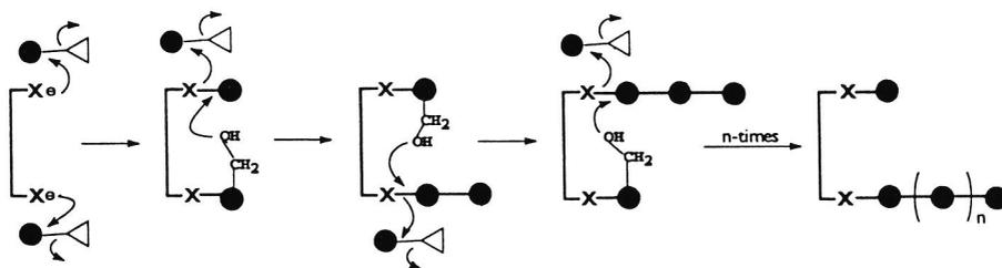
**Figure 5** Two-site insertion mechanism for the synthesis of *Ln. mesenteroides* B-512F dextran by dextransucrase. X orients the glucosyl units so that their C6 hydroxyl groups can make an attack onto C1 of the opposed glucosyl unit. X, nucleophilic group; ●, glucosyl unit, ▽, fructosyl unit. From Robyt (1996).
