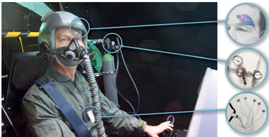
Subject flying the RNLAf ASD flight simulator, while breathing a reduced oxygen gas mixture via the (normobaric) hypoxia set-up, and being connected to sensors for measuring electrocardiography (ECG) at the chest, oxygen saturation (SpO2) at the forehead by means of pulse-oxymetry, and relative concentration changes in cerebral tissue saturation at the fronto-temporal part of the brain by means of Near InfraRed Spectroscopy (NIRS).
