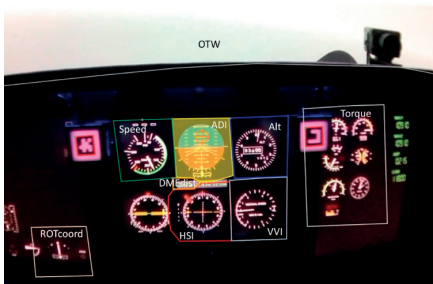
Screenshot taken from the analysis software, showing the fixation marker at the ADI in relation to the different cockpit instruments
