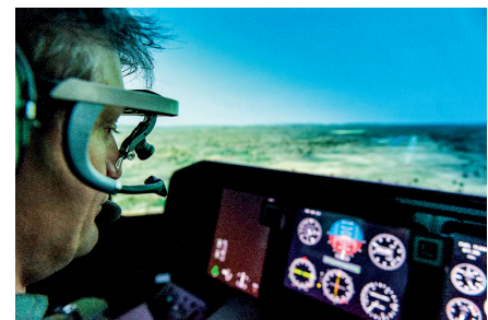
Head-mounted binocular eye tracking system to measure the viewing behavior during different phases of flight
