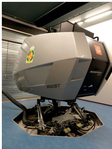
The RNLAf ASD moving-base flight simulator, located at TNO Soesterberg, The Netherlands
