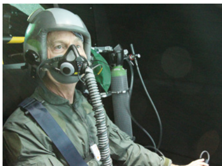
Hypoxia set-up inside the flight simulator
