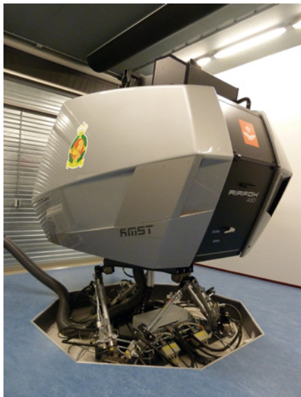
The RNLAf ASD moving-base flight simulator, located at TNO Soesterberg, The Netherlands
