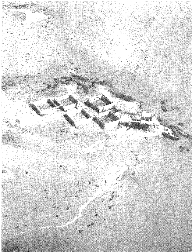
7.2 Fig. 1 Basins set up on a mussel bank for environmental toxicology tests with heavy metals (De Wolf, De Kock and Stam, 1972) (Aerial photograph — Schiphol)
