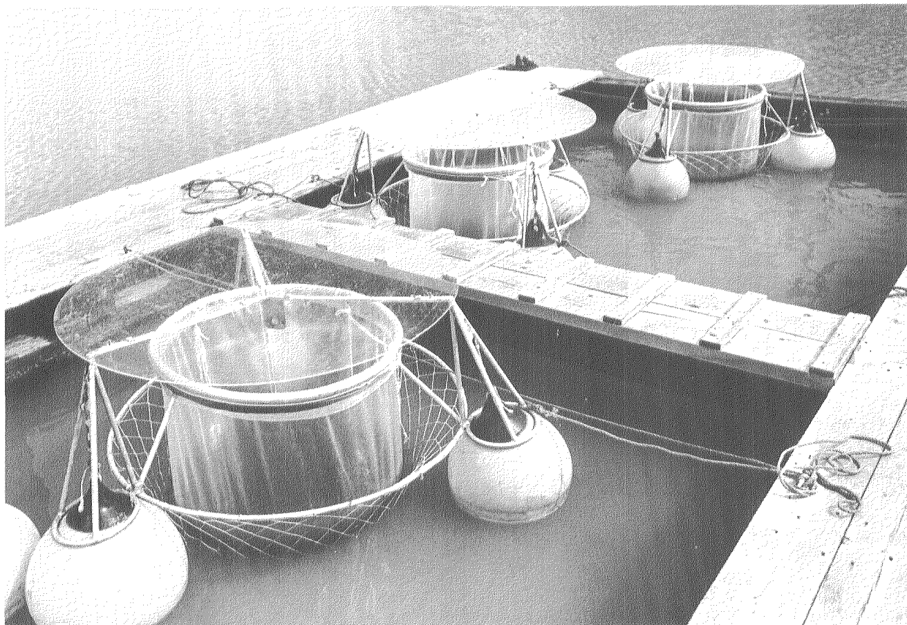
7.2 Fig. 3 Plastic bags for environmental toxicology studies on plankton populations at TNO Applied Marine Research Laboratory, Den Helder, the Netherlands (part of TNO Division of Technology for Society)
