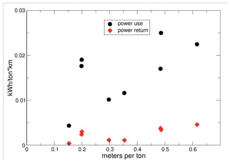
The weight of the rolling stock relative to the load transported determines whether this figure applies in all concrete situations. For a truck the weight of the load is typically 60% or less of the total weight. Due to the heavy weight of rail wagons and the associated running resistance, rail transport is not associated with lower energy consumption in the case of lighter, large-volume, low-density loads.
