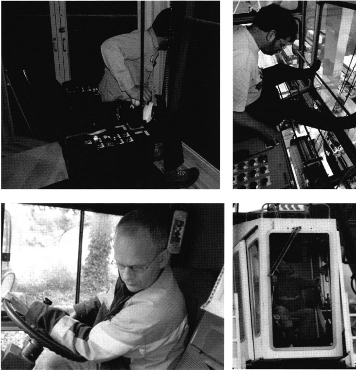
Figure 1.3 The body postures in sweeping machines, cranes, straddle carriers, which is forced by the required (near-vertical) viewing direction
