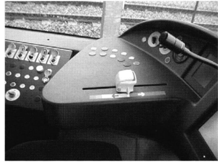
Figure 3.4 Emergency-stop, integrated in the drive-stop handle
