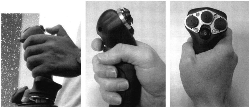
Figure 6.11 The frequently used thumb-operated switch on the joystick (left) was replaced by an index finger operated switch (middle). The foot switch was replaced by a joystick switch (right: lower middle switch)
