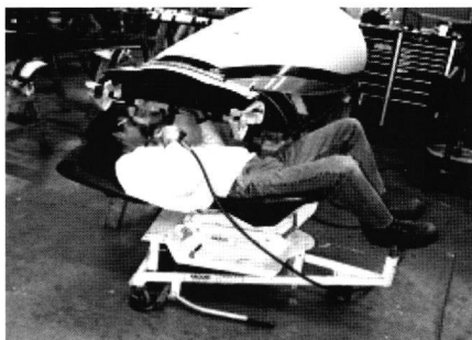
Figure 1.4 Example of an alternative body posture in the assembling industry
