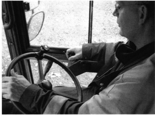
Figure 5.3 The armrest with operating system dictates the operator in a fixed position
