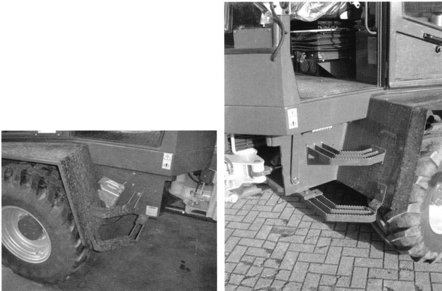
Figure 6.3 The step modification: left the old situation, right the new situation
