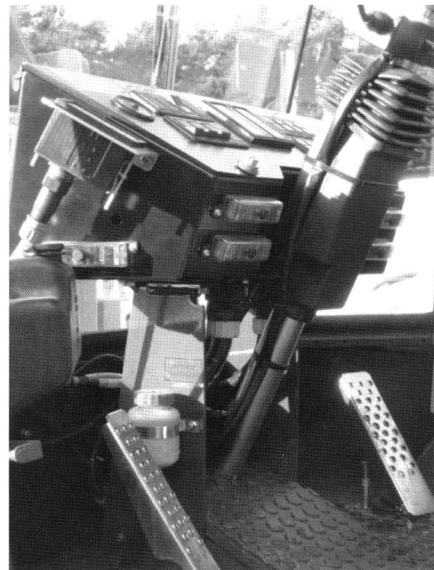
Figure 6.4 The new adjustable steering column
