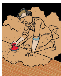
Sanding (Excenter) No control measure Excess factor: 140 times
