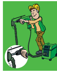
Extraction ring Prevention factor (PF): 50 – 75 times
