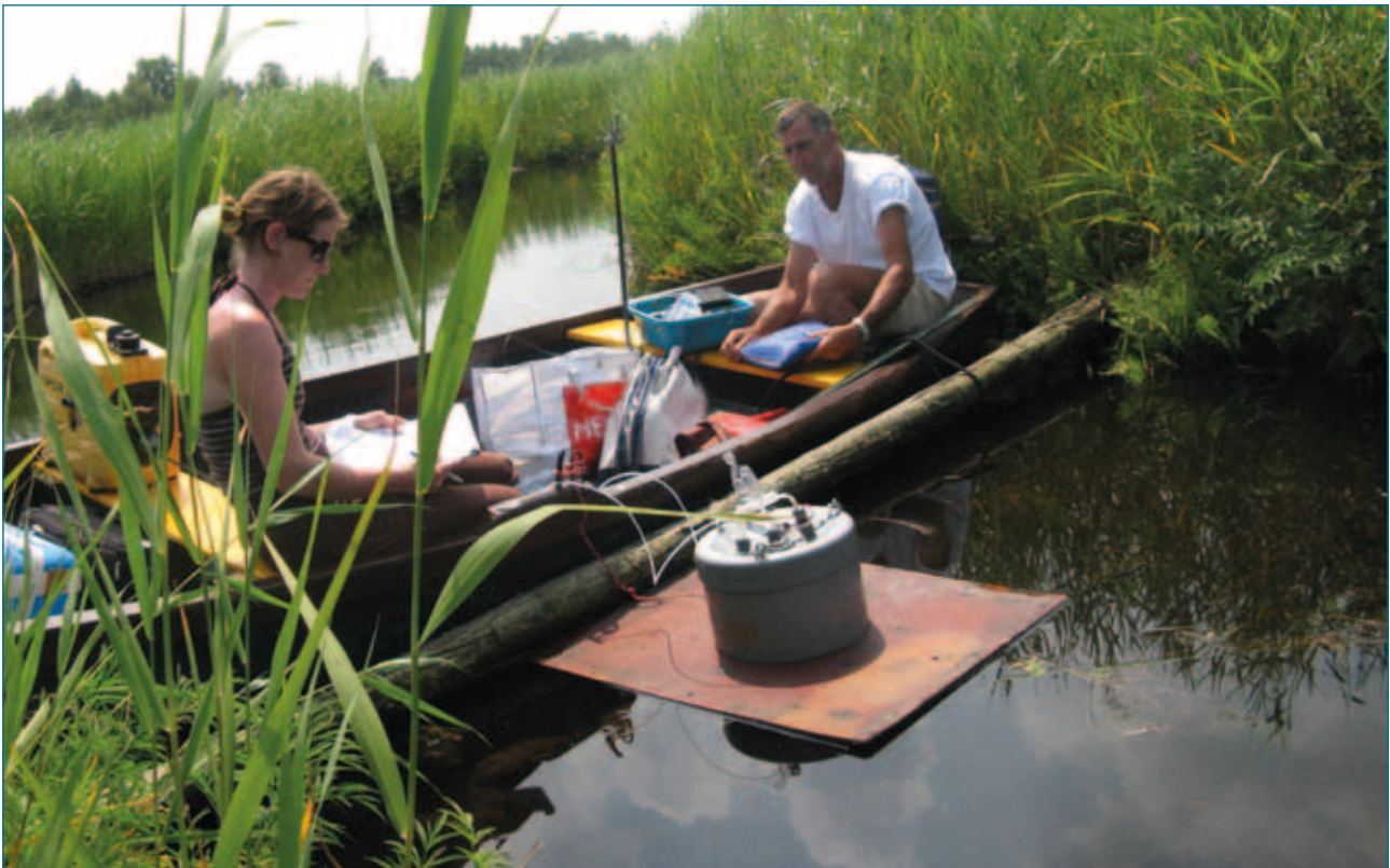
Figure 5. Chamber measurements above a ditch.
