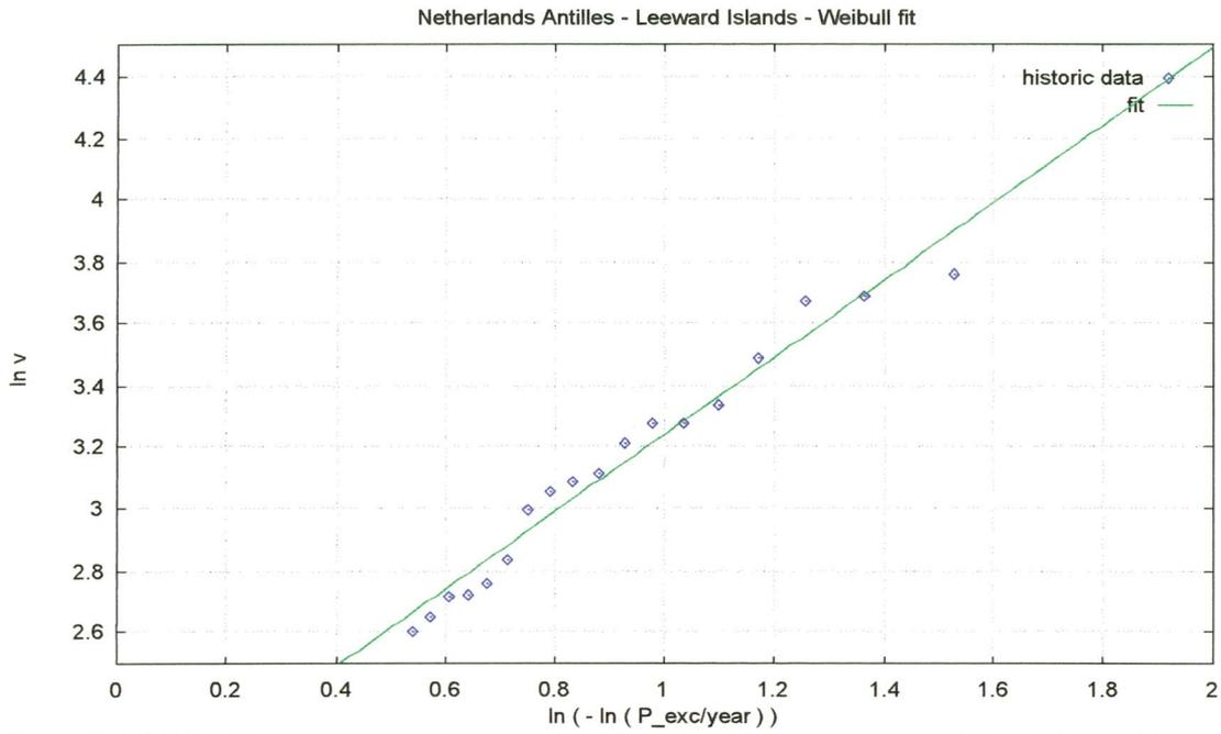
Figure 3.4: Weibull (2 parameter) fit of data on hurricane wind speeds near the Windward islands
