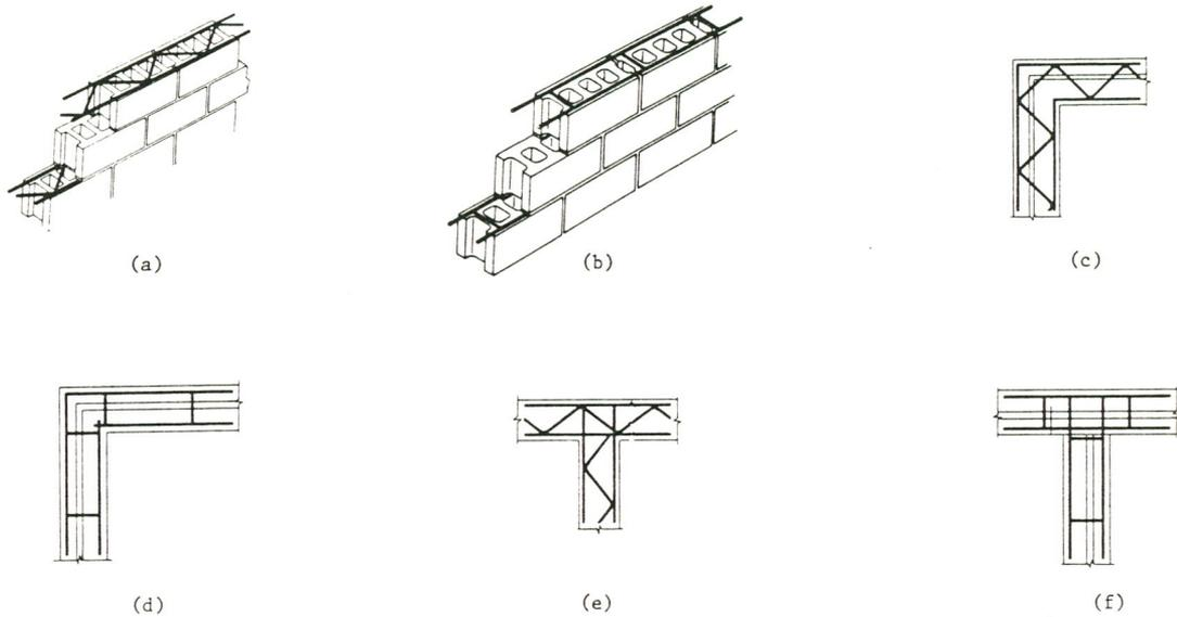
Figure 5.3: Horizontal reinforcement between intersection masonry walls: (a, b) without bond beams, (c,d) with bond beam (NBS, 1977)
