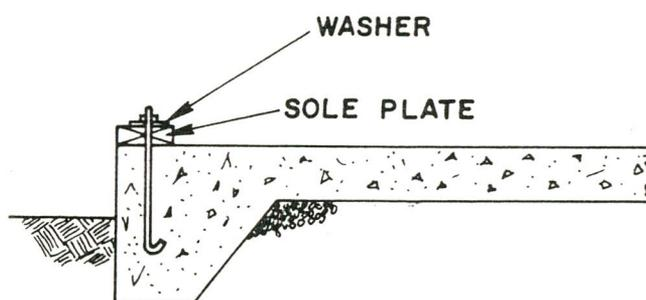
Figure 5.7: Typical timber wall construction (NBS, 1977)
