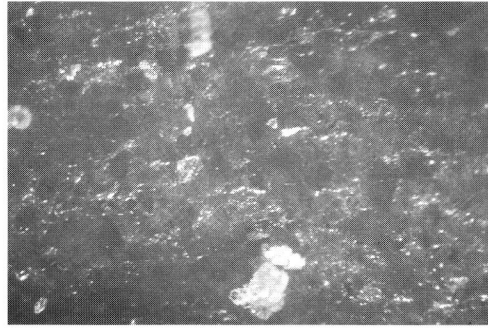
Figure 3.4: Fracture of a HNF pellet (light-microscope, diffuse lighting).
