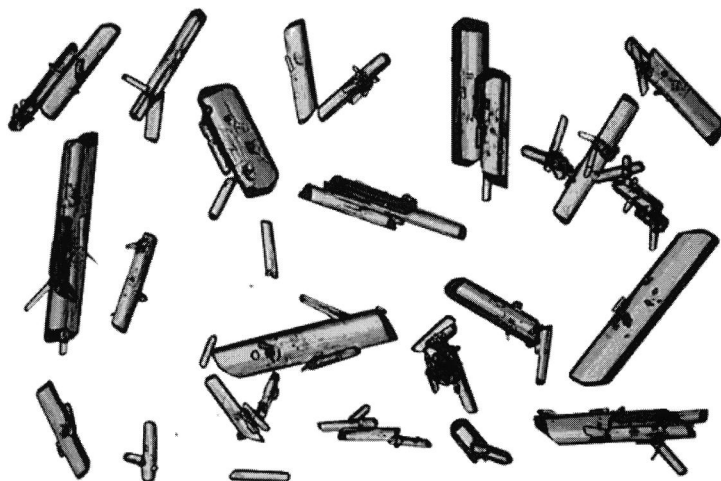
Figure 2.3: Re-crystallized HNF with length over diameter ratio's 4...5, mean diameter about 500 \mu\text{m} .
