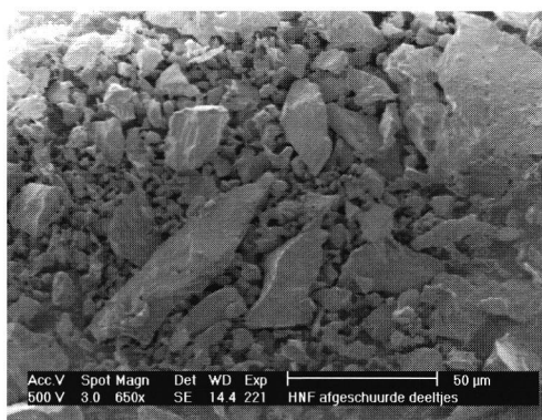
Figure 3.7: Sanded HNF (electron-microscope).
