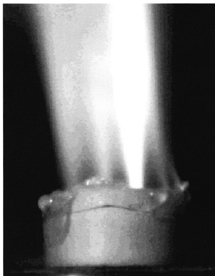
Figure 4.6: Ribbon thermocouple between two pressed HNF samples. Note the bright yellow off-center flame due to traces of sodium chloride in the HNF.
