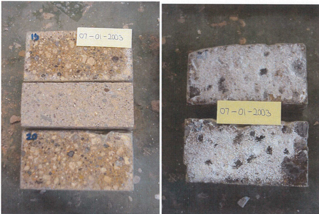
Fig. 9. Ettringen (left) and Römer (right) tuff in an accelerated salt crystallization test with \text{Na}_2\text{SO}_4 after 4 weeks (from Brendle, 2003).
