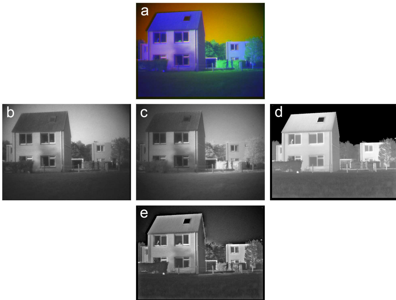
Fig 8. Example of grayscale image fusion. (a) False-color frame from series TRI_C3 with the Visual (R) channel (b), the NIR(G) channel (c) and the LWIR (B) channel (d). (e) Result of grayscale (Laplacian pyramid) fusion of (b-d). The persons behind the two upper windows in the house on the foreground (left) and the two soldiers in front of the hedge in the back are visible in different bands but are all represented in the fused image (e).
