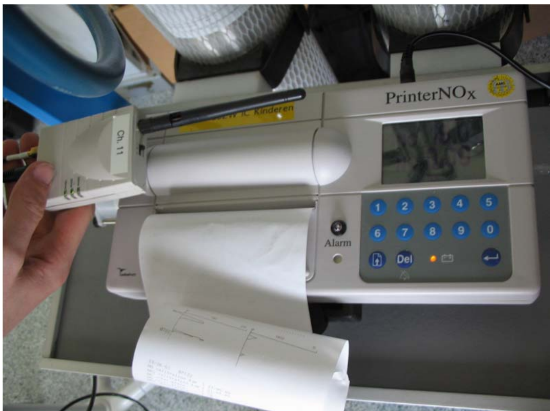
Figure C.5. WLAN antenna Ch. 11 near Printer NO x (Apparatus No. 16).
