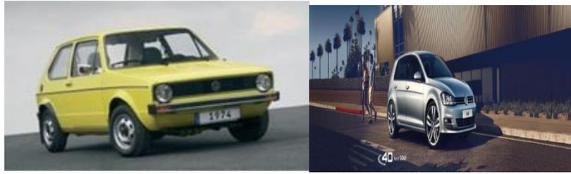
Figure 6 The current Volkswagen Golf weighs 1125-1210 kg and has a rated power of 77-90 kW, while in 1990, the weight was 855-920 kg and the power 40-66 kW.
