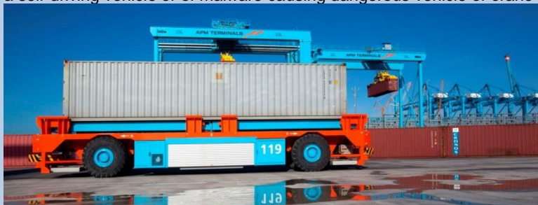
Figure 3. Automated transport vehicle at the APM terminal, Maasvlakte 2
