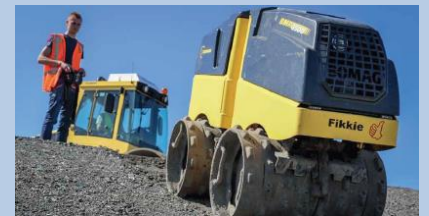
Figure 2. The remotely controllable steamroller, 'Fikkie'.
