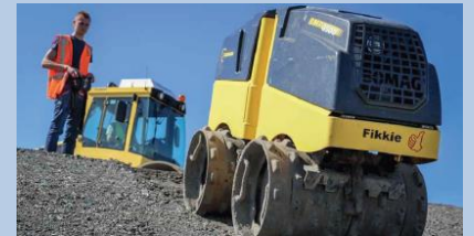
Figure 2. The remotely controllable steamroller, 'Fikkie'.
