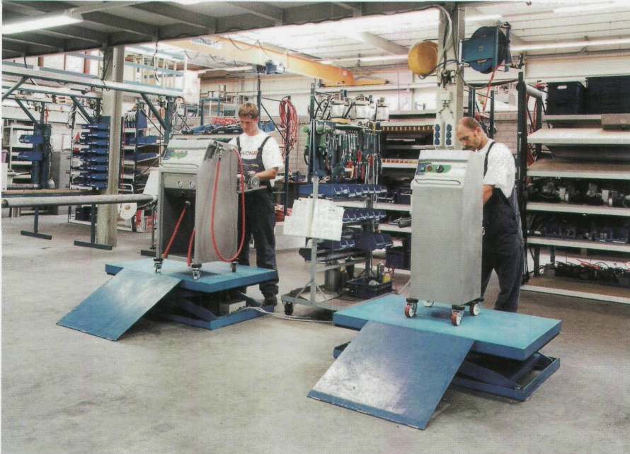
In the new situation lifting tables ensure that work can always be carried out at the correct height.
