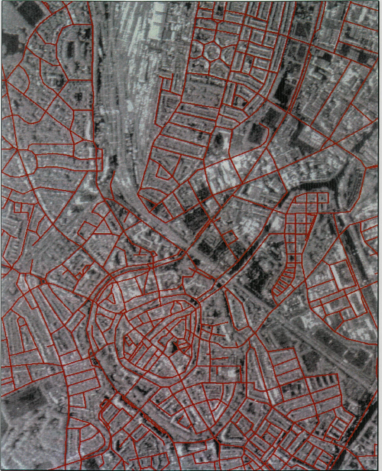
Figure 2.3-5 PHARUS image with overlay VOR data set (see text for explanation)
