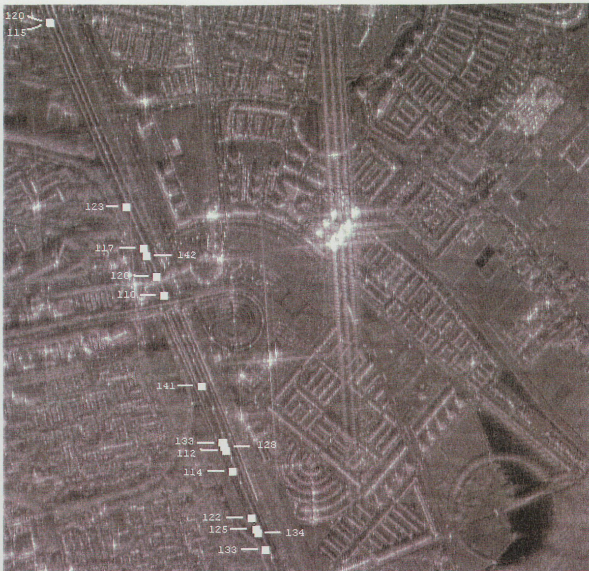
Figure 4.1-4 Composite SAR/MTI image showing moving targets on the left (in the image) side of the A12. Velocities are indicated in km/h.
