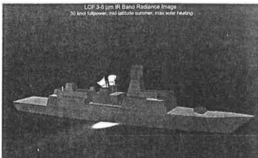
Figure 9: SHIPIR simulation of the LCF Design in the MIR-window.
