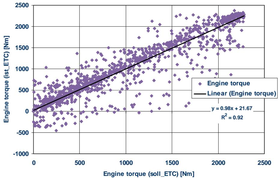
The correlation between 'soll' and 'ist' torque can also be shown over the cycle, as depicted in the figure below. It is clear that the 'ist' torque follows the 'soll' torque well but momentarily deviations may occur.
