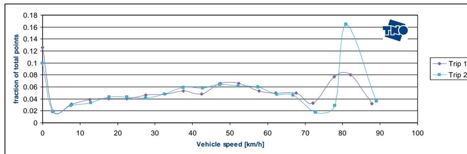
Figure 3.11: speed binned CO<sub>2</sub> emission of trip 1 and trip 2
