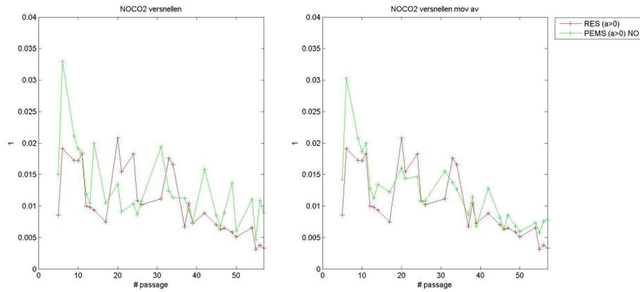
Figure 3.37: Euro IV 12t delivery truck Remote Emission Sensing (RES) data compared to PEMS data (right: moving average of 5 seconds)
