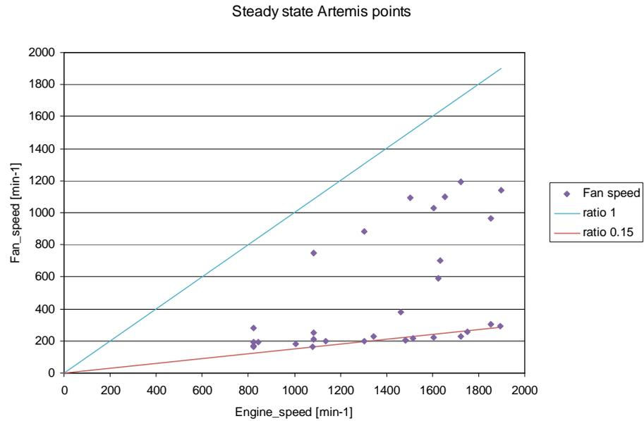
Figure 3.19: fan speed and engine speeds during the ETC, indicating the slip of the viscous clutch
