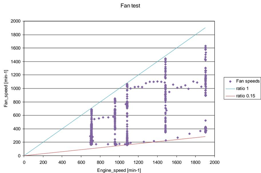
Figure 3.18: fan speed a different steady state engine speed of the Artemis test, indicating the slip of the viscous clutch
