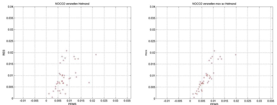
Figure 3.40: comparison of Euro IV 12t delivery truck RES and PEMS measurement data, lhs second based PEMS data, rhs 5 second moving average PEMS data
