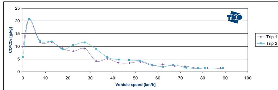
Figure 3.15: speed binned CO<sub>2</sub> specific HC emission [g/kg] of trip 1 and trip 2
