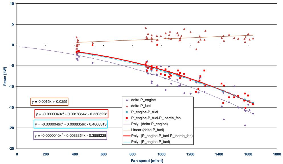
Figure 3.21: approximated absorbed total steady state fan power as a function of fan speed, including slip from the viscous clutch
