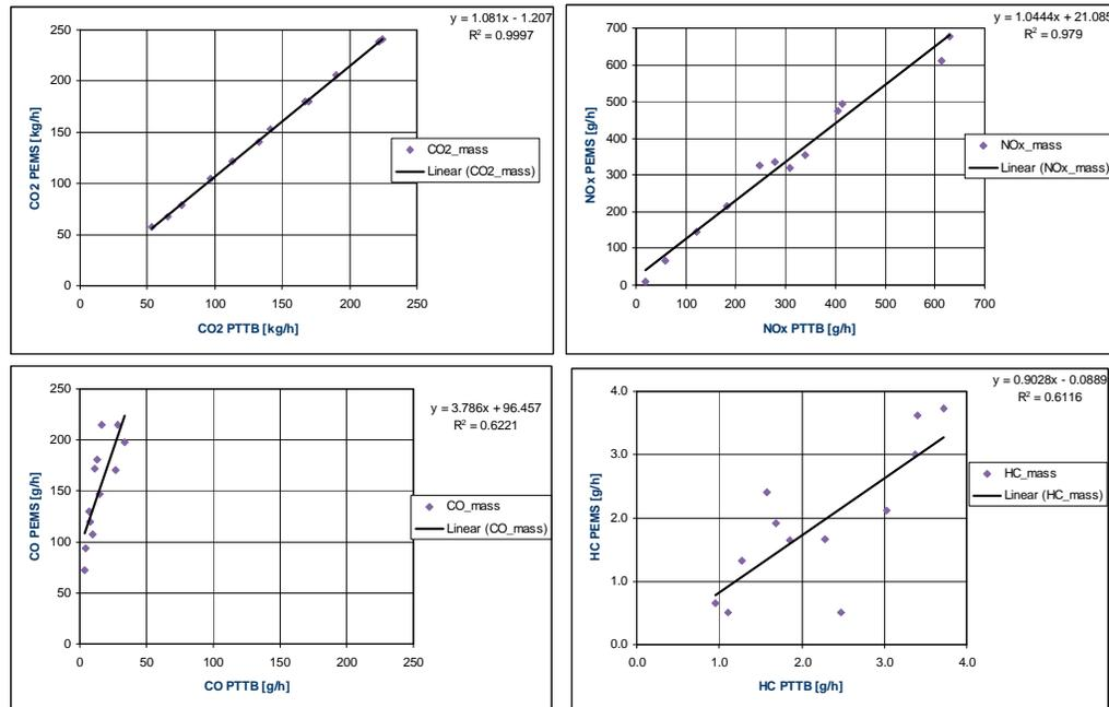
The difference between the PEMS and the PTTB was further investigated to find the cause. For both systems the mass emissions over a test cycle are determined by:
