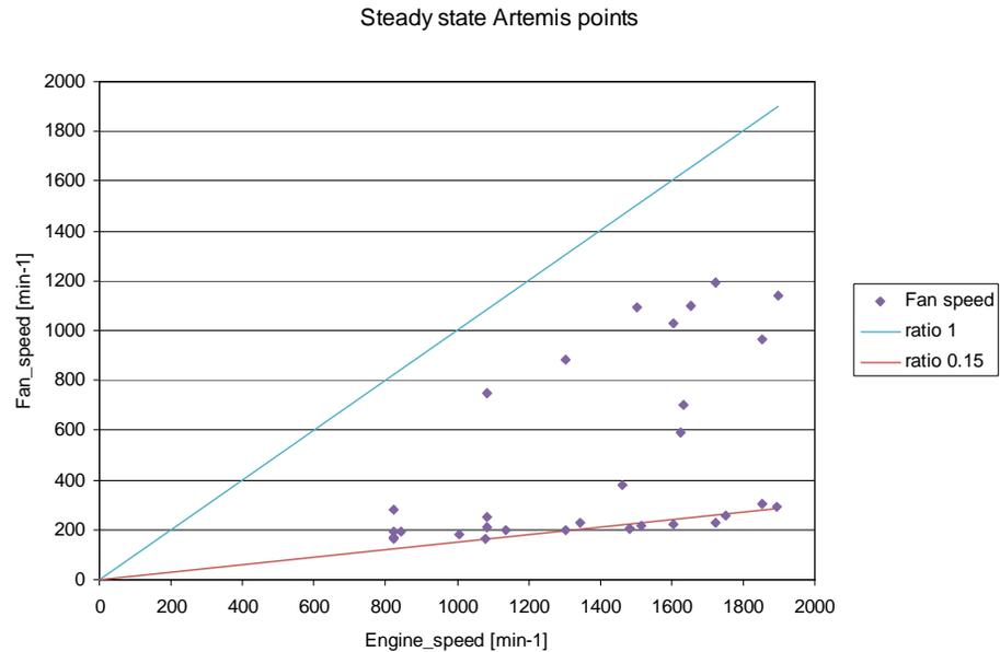
Figure 3.19: fan speed and engine speeds during the ETC, indicating the slip of the viscous clutch
