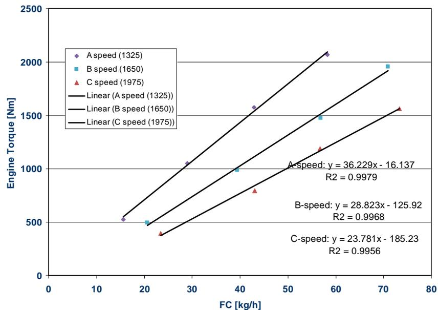
The following graph shows the calculated static drive line friction losses for a DAF XE Euro III engine mounted in a chassis with a manual gear box. The friction under load is heavily related to engine speed and only little to engine load. This means
