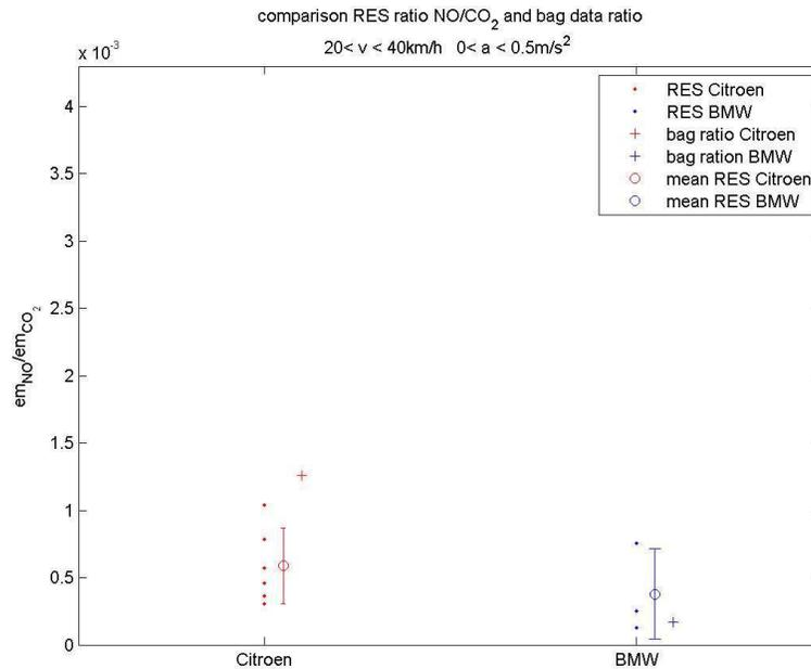
The figure shows that within this v-a bin the measured ratios for Citroën and BMW are more or less the same within the measurement error.
