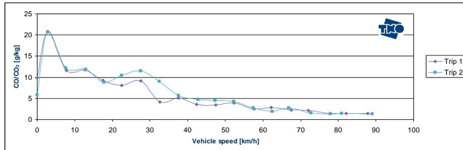
Figure 3.15: speed binned CO<sub>2</sub> specific HC emission [g/kg] of trip 1 and trip 2
