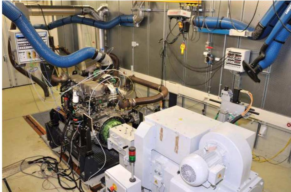
The conventional tool to test HD engines is the engine test bed. On an engine test bed an engine's crankshaft/flywheel is mounted to a dynamometer which is able to brake (or accelerate) the engine directly. Normalised torque and engine speed cycles, either steady or transient, are applied to the engine.
