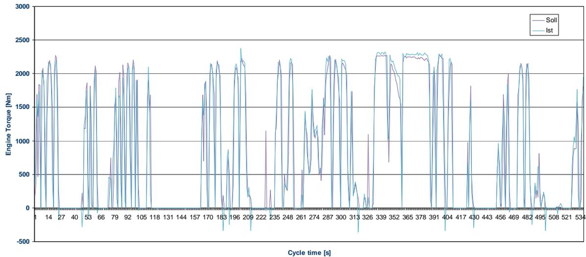
The accumulated work calculated over a test cycle is an important value as in current emission legislation limits are defined as brake specific emissions; emission per engine work delivered. The table below shows the values for the engines work determined in a few different ways; on the left the available reference values and on the right the measured and calculated values. All values are within 1%. The largest difference occurs between the repetitions of the two ETCs.
