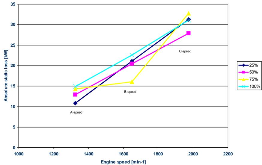
Figure 3.24: relative static friction loss of the drive line
