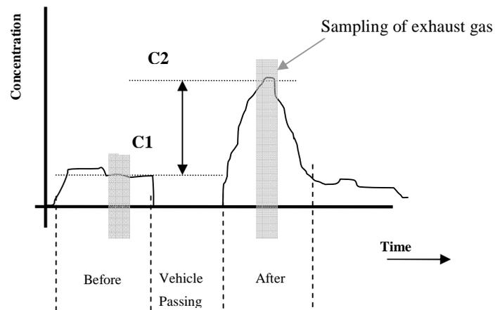
The measurement values do not represent absolute emissions of the vehicle. Only a part of the total exhaust plume is measured. The tail pipe position and meteorological conditions like wind, influence the dispersion of the gases. The measurements therefore represent the amount (number of molecules) of gases in the path of the measurement beam (no concentrations). Based on the measurements of the RSD4600 system, three separate gas ratios can be calculated:
