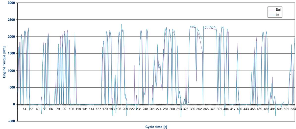
The accumulated work calculated over a test cycle is an important value as in current emission legislation limits are defined as brake specific emissions; emission per engine work delivered. The table below shows the values for the engines work determined in a few different ways; on the left the available reference values and on the right the measured and calculated values. All values are within 1%. The largest difference occurs between the repetitions of the two ETCs.
