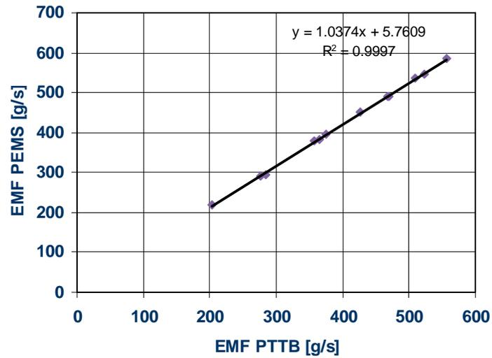
Over a transient test (ETC) the slope of the instantaneous EMF is also at about 4%.
