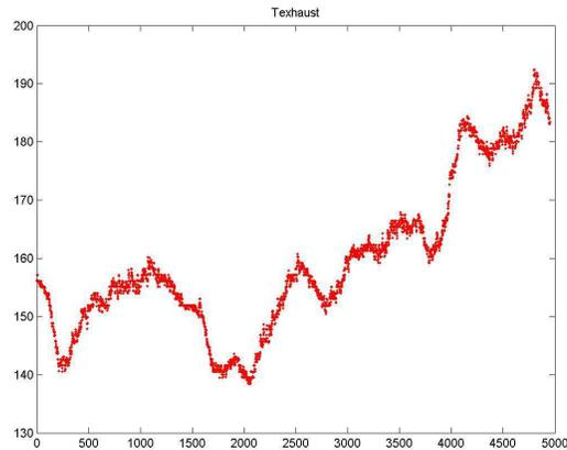
The Euro IV 12t delivery truck is equipped with EGR emission reduction technology, which efficiency depends less on exhaust gas temperature than the SCR technology of the Euro V tractor.
