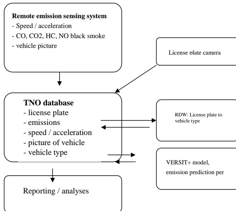
The data flow is visualized in the Figure above. The data of the RES measurements is collected in a database, this database contains following information for each single vehicle:
